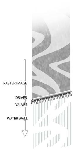
Creation of a modern, digital Water Wall by computer-controlled solenoid valves.
