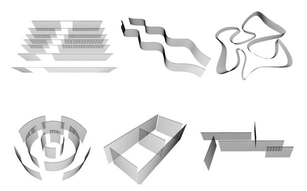
Some possible configurations of Water Walls: layers and enfilade, allée, closed loop, room plans, and free plan.
