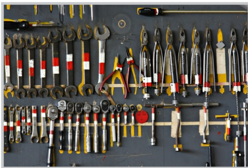
Figure 4 – Shadow board showing one pair of pliers is missing. Source: www.Plasteel.az
