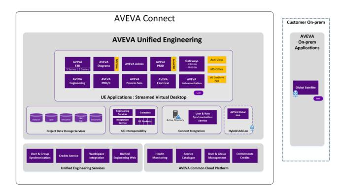
The service architecture adheres to a separation of concerns principle where each AVEVA server component is deployed on dedicated virtual infrastructure instance(s). The associated client software needs to be located on accessible virtual desktops delivered using the WorkSpaces service.
