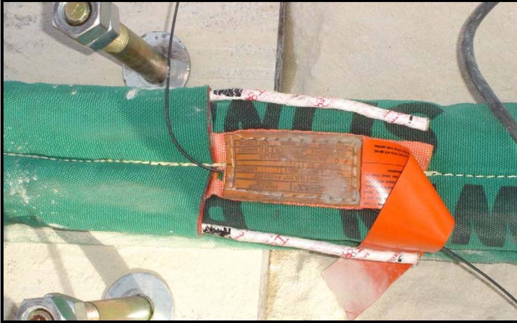
Figure 17. Inspect Slings to Determine if Tell-Tales are Visible
