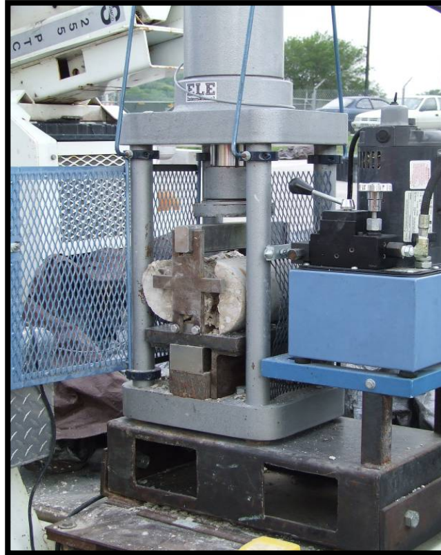
Figure 3-11. Portable Split Tensile Tester
