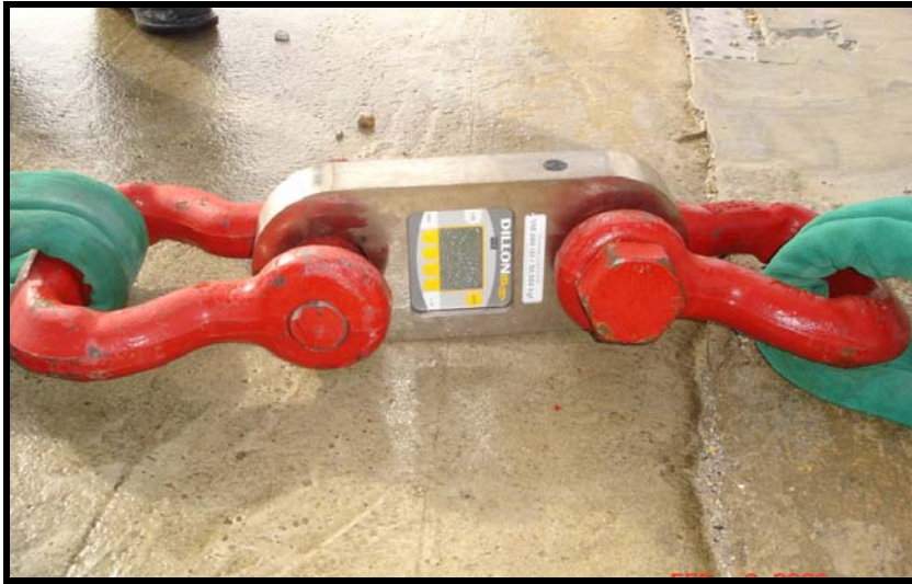
Figure 2. Load Cell Connected to Slings with 2 Shackles
