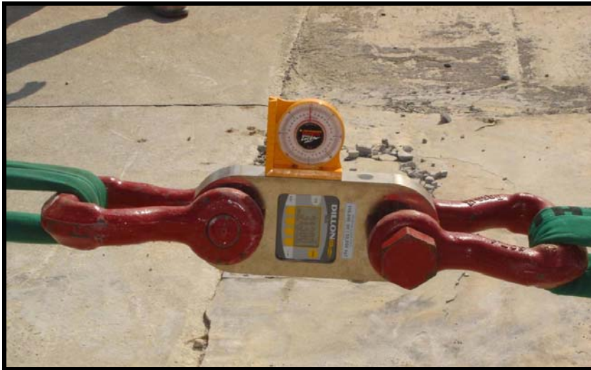
Figure 16. Magnetic Inclinometer Mounted to Load Cell
