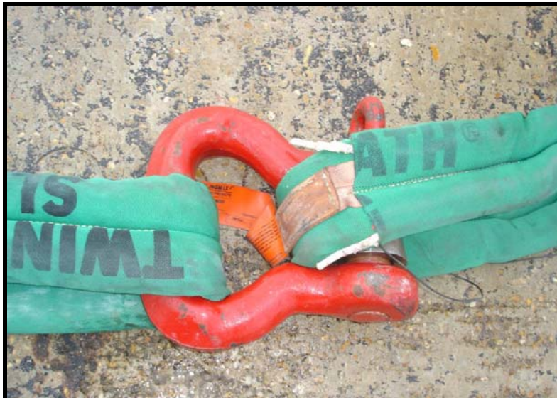
Figure 3. Slings Connected by Shackle
