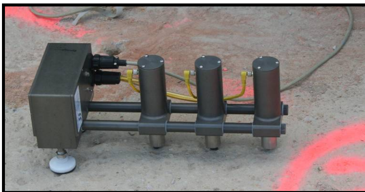
Figure 1. Portable Seismic Property Analyzer (PSPA)
