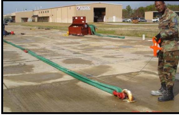
Figure 12. Measuring Distance from Anchor to Anchor Plate
