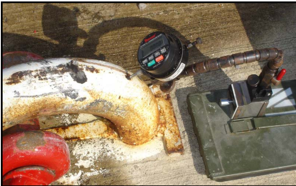
Figure 15. Mount Digital Indicator to Anchor at 45 Degree Angle
