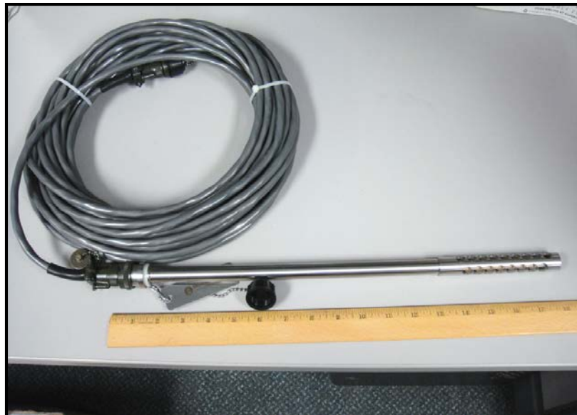
Figure B-15 Example of an ER Probe
