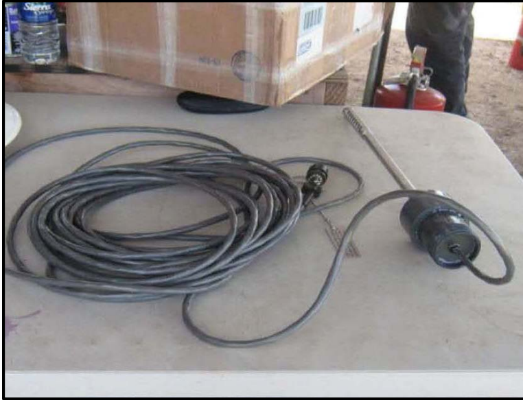
Figure B-16 Probe with Encapsulated Connector.
