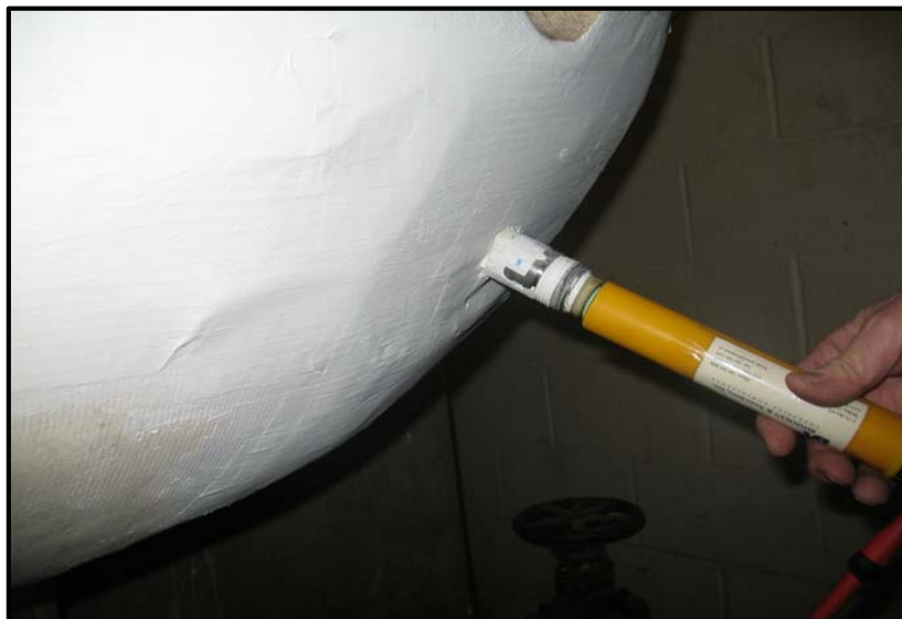
Figure B-37 Reference Electrode Placed in Contact with Moist Wadding Temporarily Placed Inside of the Capillary Tube Monitoring Port.
