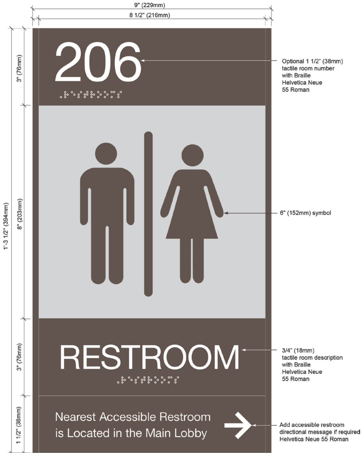
1\1 Figure 4-5 Non-Accessible Restroom Identification Signs. /1/
