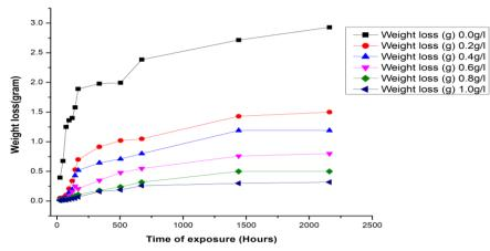
**Fig. 4:** Weight loss against time of mild steel in 1M HCl with PAPE inhibitor and without PAPE (0.0g/l) after 2160 hours of exposure
