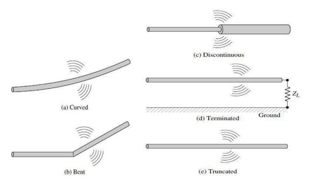
Figure: Wire Configurations for Radiation
