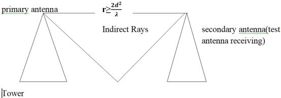
Fig:5. 8.Experimental set up for antenna test
