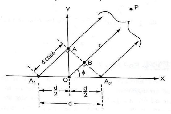
Broadside array with two isotropic point sources with equal amplitude and phase
