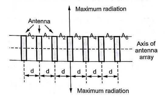
Figure - Broadside array of antennas
