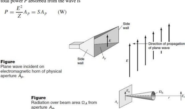
Thus, the electromagnetic horn may be regarded as having an aperture, the total power it extracts from a passing wave being proportional to the aperture or area of its mouth. But the field response of the horn is NOT uniform across the aperture A because E at the sidewalls must equal zero. Thus, the effective aperture  $A_e$  of the horn is less than the physical aperture  $A_p$  as given by
