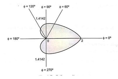
Problem 3: A broadside array of identical antennas consists 8 isotropic radiators separated by distance X/2. Find radiation field in a plane containing the line of array showing directions of maxima and null.
