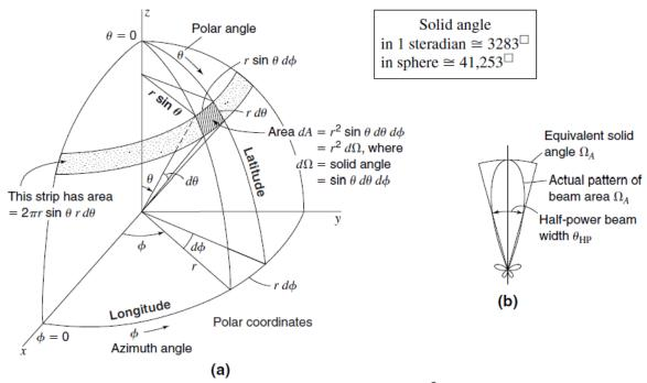
Polar coordinates showing incremental solid angle  $dA = r^2 d\Omega$  on the surface of a sphere of radius r where  $d\Omega =$  solid angle subtended by the area dA. (b) Antenna power pattern and its equivalent solid angle or beam area  $\Omega_A$ .
