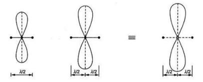
Radiation pattern of 2-element array with amplitude ratio 1:2:1.
