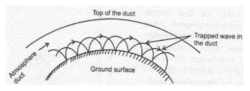
Fig. 4.10 Duct Propagation
