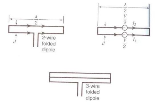
The input impedance for a dipole is 73  $\Omega$ . Hence for a folded dipole with 2 arms the radiation resitance is  $2*73\Omega = 292\Omega$ . If 3 arms are used the resistance will be  $3^2*73\Omega = 657\Omega$
