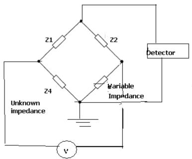
Fig: 5.1. Wheat stone Bridge for impedance measurement
