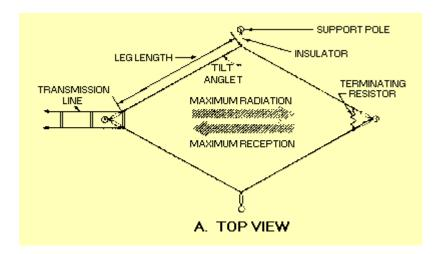
The rhombic antenna is widely used for long-distance, high-frequency transmission and reception. It is one of the most popular fixed-station antennas because it is very useful in point-to-point communication.
