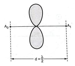
Field pattern for two point sources with equal amplitude in-phase current
