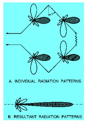
Figure a. shows the individual radiation patterns produced by the four legs of the rhombic antenna and the resultant radiation pattern. The principle of operation is the same as for the V and the
