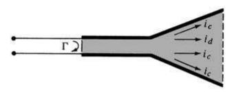
(b) Reflection, conduction, and dielectric losses
