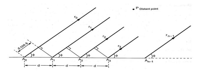
The electric field produced at point P due to an element A<sub>0</sub> is given by,
