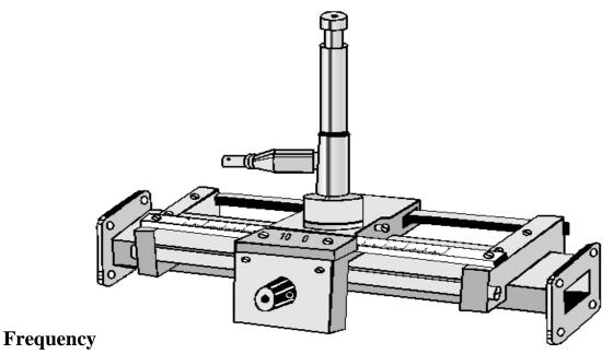
Fig: 3.Prespective view of slotted line arrangement
