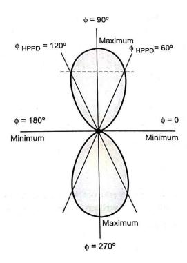
Field pattern for two point source with spacing  $d = d = \frac{\lambda}{2}$  and fed with currents equal in magnitude and phase
