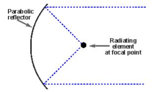
Diagram of a focal feed parabolic reflector antenna
