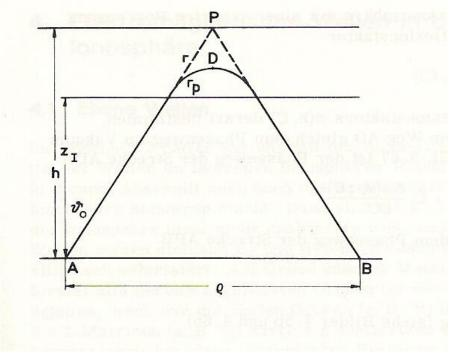
Fig: 10 Vertical incidence measurements of the ionosphere
