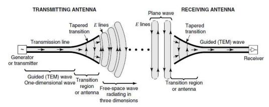
An antenna is basically a transducer. It converts radio frequency (RF) signal into an electromagnetic (EM) wave of the same frequency. It forms a part of transmitter as well as the receiver circuits. Its equivalent circuit is characterized by the presence of resistance, inductance, and capacitance. The current produces a magnetic field and a charge produces an electrostatic field. These two in turn create an induction field.
