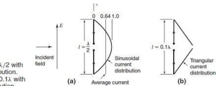
**Figure**(a) Dipole of length  $I = \lambda/2$  with sinusoidal current distribution.
