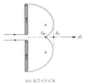
When  $l > \lambda$ , the current goes phase reversal between adjoining half-cycles. Hence, current is not having same phase along all parts of transmission line. This will result into interference and canceling effects in the total radiation pattern.
