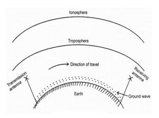
Fig 4.1 Ground wave Propagation
