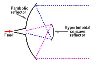
Diagram of a Gregorian feed parabolic reflector or dish antenna
