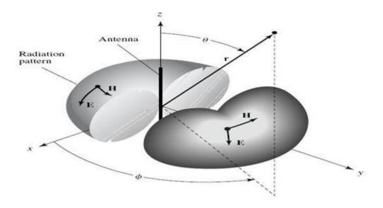
Fig. Omnidirectional antenna pattern
