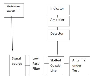
Fig5.4.Block diagram of making slotted line measurement
