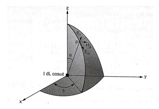
Electromagnetic field at point P when an alternating current element IdL cosot placed at origin
