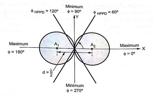
Field pattern for two point sources with spacing  $d=\frac{\lambda}{2}$  and fed with currents equal in magnitude but out of phase by  $180^{0}$
