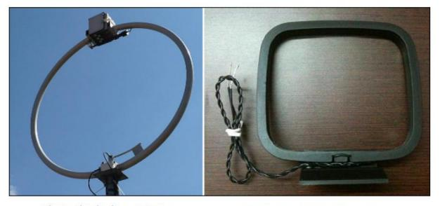
Fig 1: Circular loop antenna
