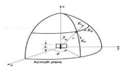
Fig:5.5 Spherical coordinate system for pattern measurement XY-Plane is horizontal plane and XZ-plane is vertical plane the radiation pattern is
