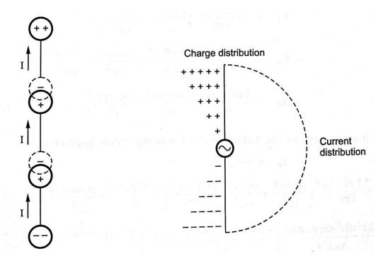
Chain of Hertzian dipoles and charge and current distributions on linear antenna
