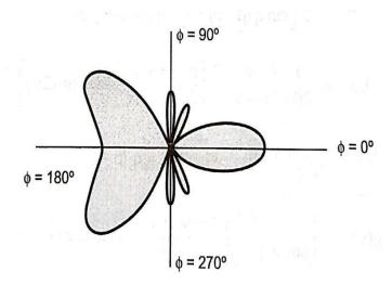
field pattern for 4 element end fire array with equal amplitude and  $\frac{\lambda}{2}$  spacing for increased directivity
