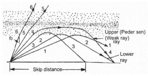
Fig 4.4 Effect of ionosphere on rays
