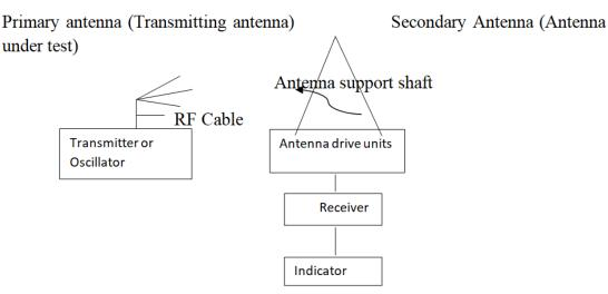
Fig:5.6.Radiation pattern measuring set up
