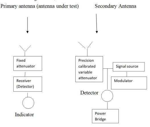
Fig:5.9 Set up for Gain measurement by comparison method
