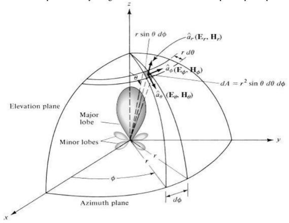
Fig. Coordinate system for antenna analysis
