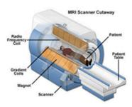
When your body is scanned you lie on a horizontal platform, which carries you inside the machine into a set of coils. These coils produce a magnetic field, which affects the protons in the hydrogen atoms in the water molecules in your body. These are then agitated by the radio signals and the responding radio signals from the protons are detected by the scanner, and processed into an image. This image is then used by doctors to help with diagnosis.
