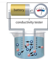
Figure 2.39 An aqueous solution of an ionic compound will conduct electric current because the ions are free to move toward the oppositely charged electrode.
