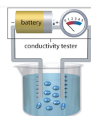
Figure 2.40 If a molecular compound is polar, the positive end will orient toward the negative electrode and the negative end will orient toward the positive electrode. A non-polar molecule will be induced to form a dipole. However, the charges cannot leave the molecule and thus no electric current will flow.
