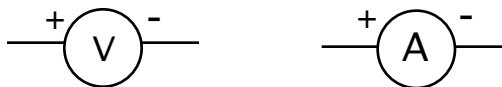
Figure 3-6: Symbols for a voltmeter (left) and an ammeter (right). The + sign on the voltmeter should be at the higher potential if the voltmeter reads positive. If the current in the ammeter flows from + to – then the ammeter reads positive.
