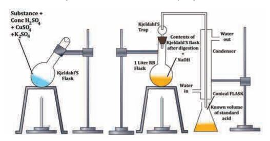
Fig 11.3 Kjeldahls method
