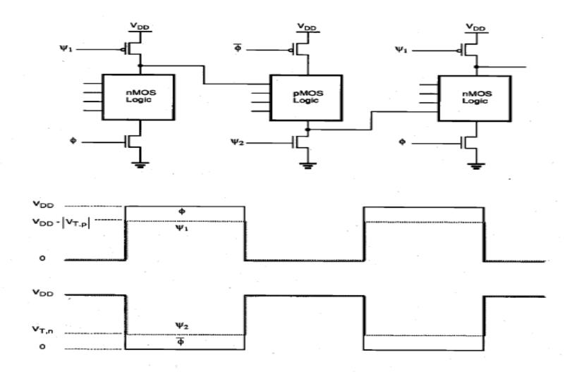
Fig. General circuit structure and the clock signals of Zipper CMOS
