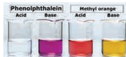
Figure 6.4 Test for acid and base using indicator
