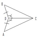
39. Tony is surveying. He starts at point A and sites point D. He measures a 50° angle between point D and a new point C. He measures 30' to point C. At point C, he turns and measures 40' towards the line between A and D. He places a stake at point B. If he were to come back to point A with the same measurements and orientation, would he be able to find the Corner D? Why or why not?
