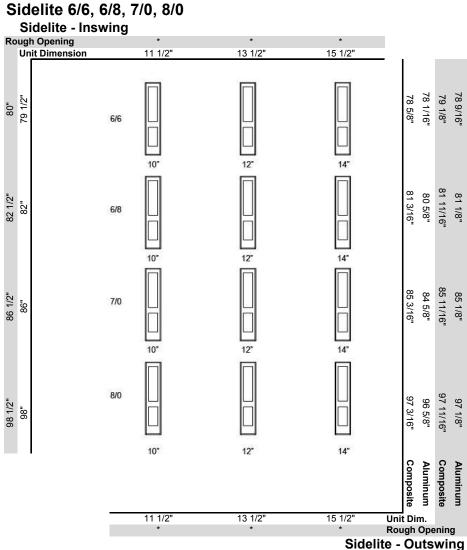
\*Add actual unit dimension to <u>door</u> rough opening width for <u>total</u> rough opening width.
