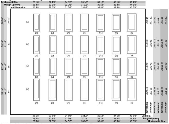
\*For M.E.U., add actual unit dimension to <u>door</u> rough opening width for <u>total</u> rough opening width.
