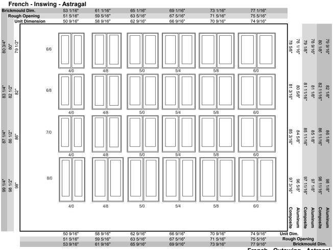
For units with public access sills, subtract 1" from inswing height. Unit widths will be the same as in the table above.
