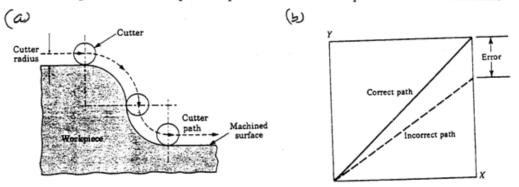
Figure 5. (a) Continuous path cutting and (b) Position error caused by the velocity error
