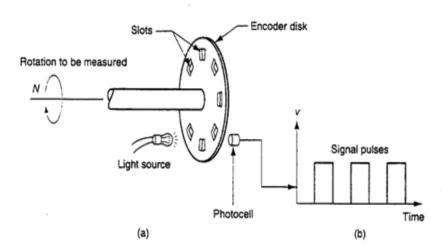
Figure 11. Optical Encoder (a) Device (b) Series of pulses emitted
