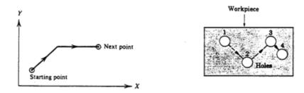
Figure 4. Cutter path between holes in a point-to-point system
