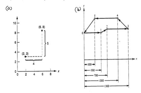
Figure 8. (a) Absolute versus incremental; In absolute positioning, the move is specified by x = 6, y = 8; in incremental, the move is specified by x=4, y=5 for the tool to be moved from (2,3) to (6,8)
