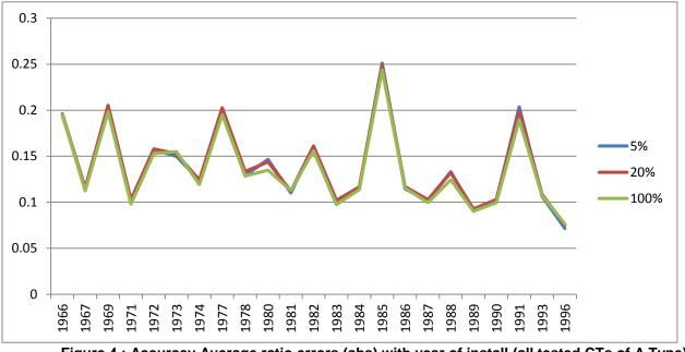
Figure 4 : Accuracy Average ratio errors (abs) with year of install (all tested CTs of A Type)
