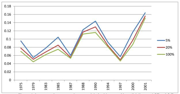
Figure 6 Accuracy Average ratio errors (abs) with year of install (all tested CTs of C Type)
