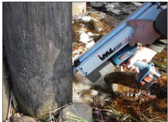
Figure 2.11—Drilling can take place at an angle to assess the area below ground line.
