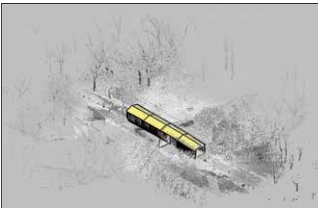
Figure 4.10—3D AutoCAD image of the Cedarburg Bridge embedded in point cloud data (SightLine, LLC).
