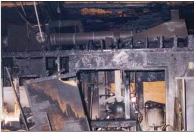
Figure 5.3—Area of fire origin in Building 2 fire at the Forest Products Laboratory.
