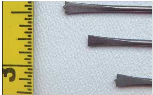
Figure 2.10—Flat-tipped resistance drill bits used to inspect timber materials.
