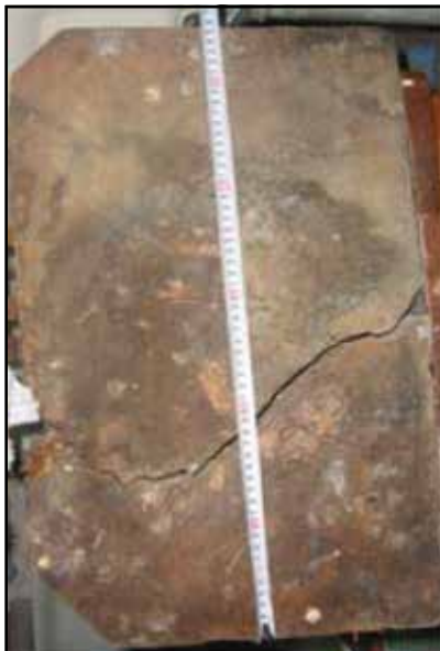
Figure 4.4—Acoustic tomogram revealed internal crack of an old timber at the Imperial Palace in Beijing (Yu et al. 2009).
