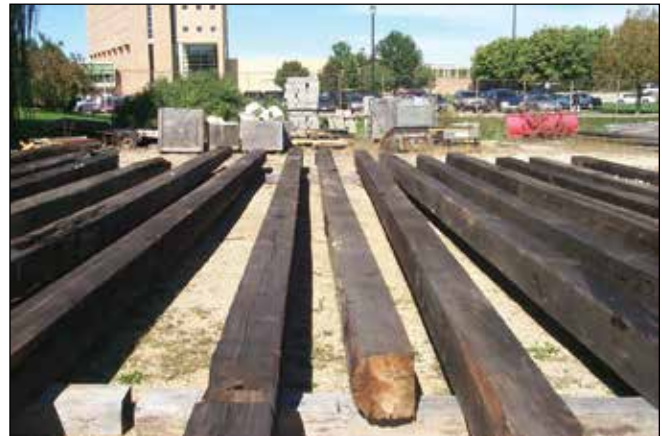
Figure 7.1—Fifteen 12- by 12-in. white pine timbers removed from the Quincy Mine Blacksmith Shop.
