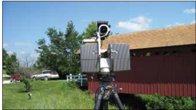
Figure 4.8—A FARO laser scanner used to scan a historic covered bridge.
