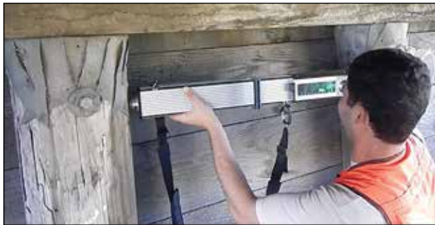
Figure 2.13—Electronic display on a resistance drill.
