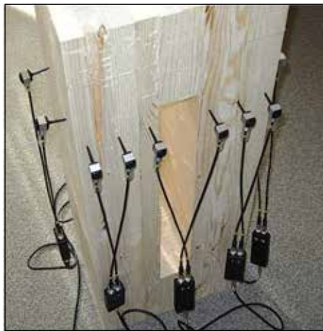
Figure 4.3—Acoustic tomography test on a glued-laminated specimen with a simulated void (Divos 2006).
