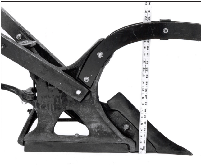
Figure 7—Vulcan plow showing about 1\frac{1}{4} inch of bottom suction.
