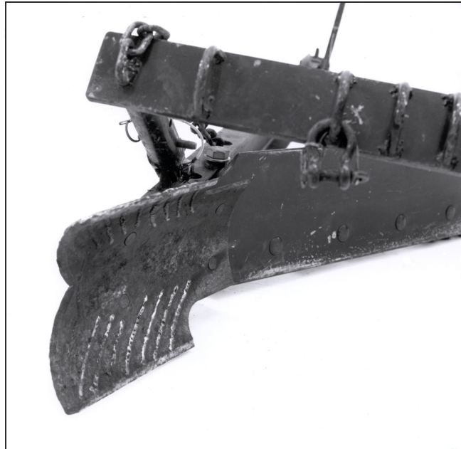
Figure 34—Blade on the MTDC combination plow and grader, fabricated from well casing.
