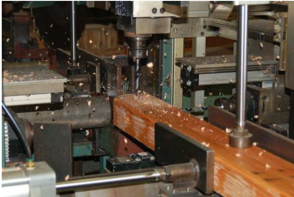
A computer-controlled drilling machine places holes into a wooden power line crossarm.
