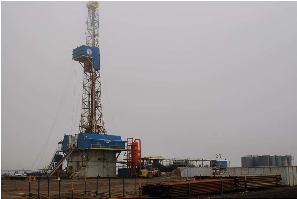
Oil well drilling rig in the Bakken oil play (Stanley, North Dakota). These rigs drill approximately 2 miles down, then drill horizontally and fracture the shale rock to allow oil to seep out and be collected.
