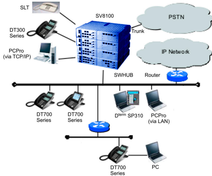
Figure 1-7 Simplified SV8100 System (9.5" Base and Expansion) Connectivity
