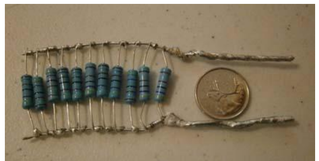
Figure 2 Practical Design of Home- Brew Termination Resistor
