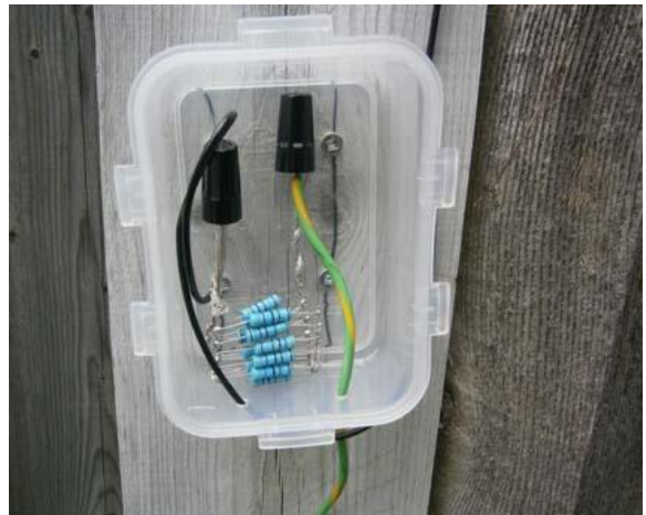
Figure 14 Termination Resistor of Beverage Antenna in Open Plastic Food Box
