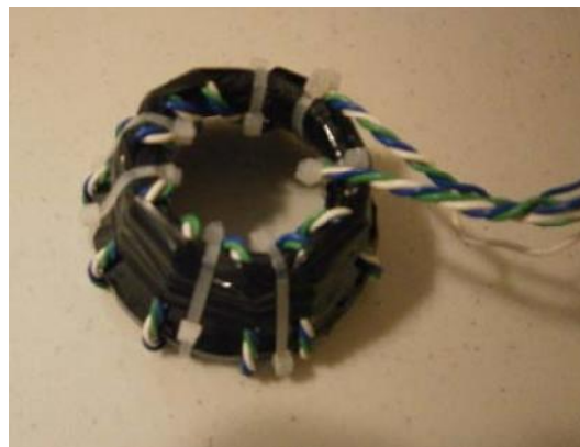
Figure 7 Unsymmetrical RF Transformer 1:9 on TV Yoke
