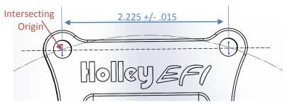
Figure 8: Marking the mounting plate for bracket mounting hole drilling
