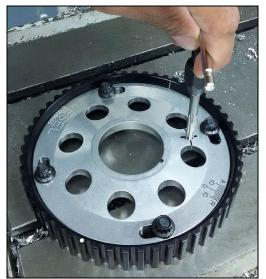
Figure 12: Tapping the Cam Hub
