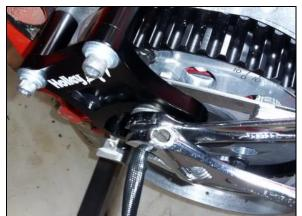
Figure 15: Locking Sensor Gap & Position
