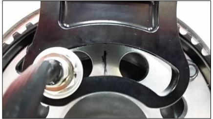
Figure 9: Angular Reference Marking
