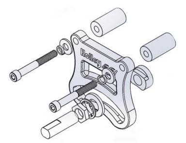
Figure 2: Sensor Bracket Assembly
