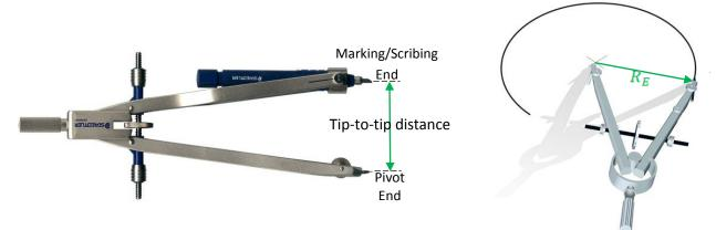
Figure 6: Drafting compass anatomy & tip-to-tip distance.
