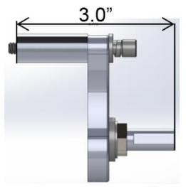
Figure 1: Bracket Assembly Standoff
