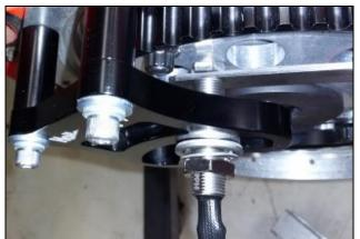
Figure 14: Adjusting Sensor Gap
