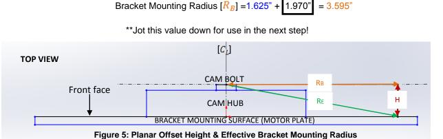
3. Use a set of calipers to measure the *Planar Offset Height* [H] for the application (**Figure 5**). This is defined as the difference in height from the <u>exact</u> surface/plane which contains the camshaft's centerline [ $C_L$ ], to the front face of
