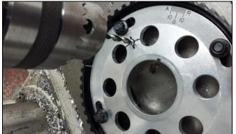
Figure 11: Drilling the Cam Hub.
