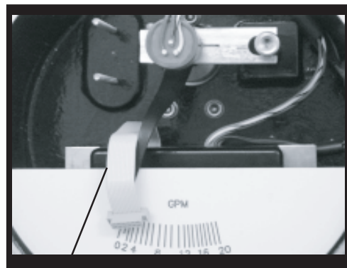
Fig. 12B Close up of Ribbon Cable for Connection to Remote Programmer in a R Box
