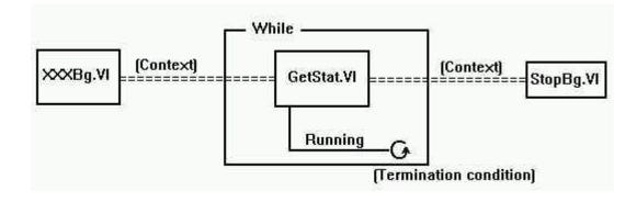
Figure 4-1. Background VIs General Wiring Pattern
