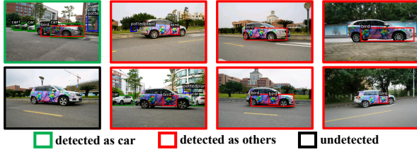
Figure 7. The results of attacking Volvo XC60 (top row) and Volkswagen Tiguan (bottom row). The generated camouflage patterns fool detectors to misrecognize the car as bird.
