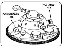
b. Attach the pool return hose (inlet of pool) to the pool return port on the tank cover.
