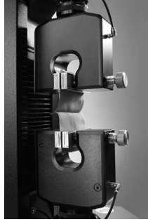
Seam Slippage Test (T27)
