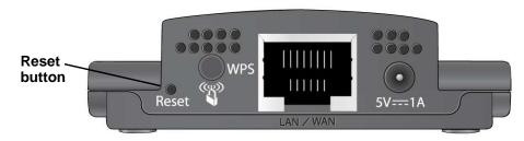
Figure 6. The Reset button restores factory settings
