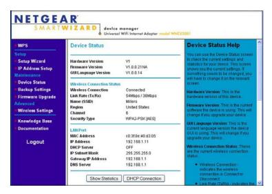
The Device Status screen shows what the current settings are for the Internet adapter. A menu in the left pane allows you to view or change the settings.
