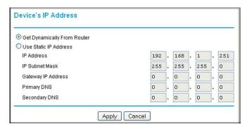
This screen shows whether the Internet adapter is set to get its IP address dynamically from the router (this is the most common setting), or is set as a static IP address.
