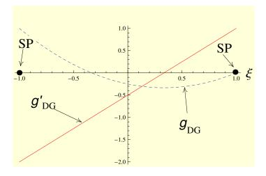
Figure 10 – Correction function  $g_{DG}$  and its derivative  $g'_{DG}$ , for n = 1.
