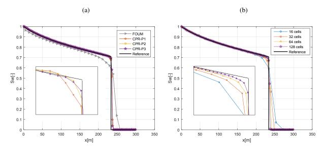
Figure 21 – Buckley Leverett problem for t=1,500 days (a) p-refinement and (b) h-refinement.
