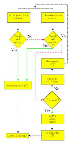
Figure 14 – Flowchart of the hierarchical MLP limiting procedure, solid green line  $\rightarrow$  if criteria is satisfied, and dashed red line  $\rightarrow$  else.
