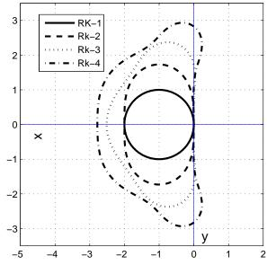
Figure 18 – Stability regions of the Runge-Kutta method in the complex  $\Omega\Delta t$ -plane, from 1 to 4 stages.
