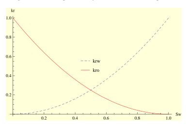
Figure 2 - Relative permeability functions for water-oil phases.
