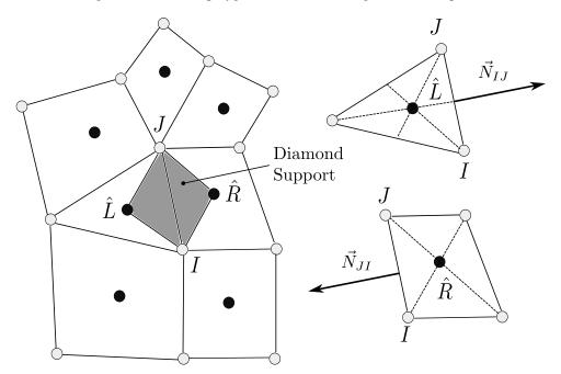
Figure 37 – Part of a polygonal mesh, illustrating the diamond path.
