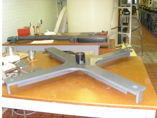
b) Bottom of the string rack with the borehole seat.
