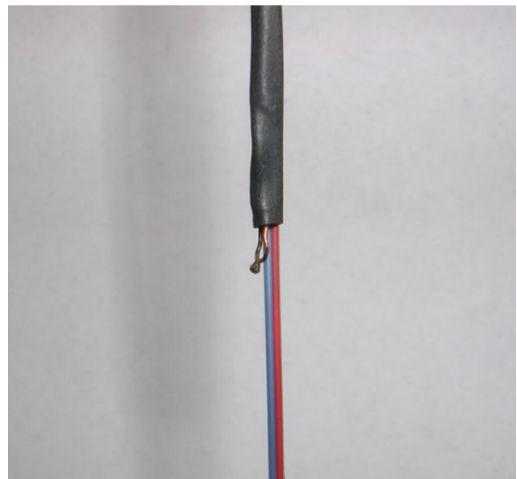
c) Thermocouple fixed on the fishing wire with a shrink tube.
