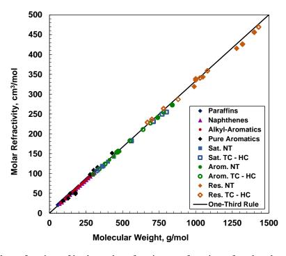
Figure G-1. Molar refraction of hydrocarbon fractions as function of molecular weight.
