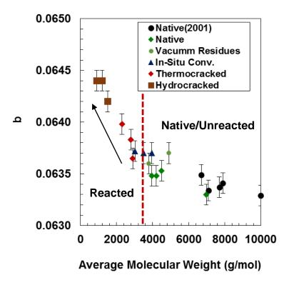
**Figure 5-36.** Fitted parameter b as function of the average aggregated molecular weight of asphaltenes at 50°C. Note that the error bars come from the sensitivity analysis explained in section 5.4.2.
