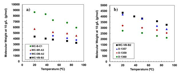
**Figure 5-16.** Molecular weight of asphaltenes at 10 g/L as function of temperature for asphaltenes from a) native and b) thermocracked oil samples.
