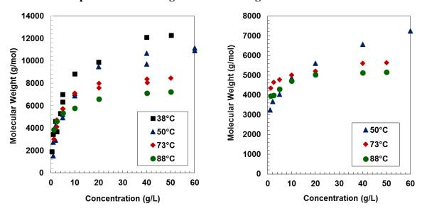
**Figure B.1**. Effect of temperature on molecular weight measurements for C7-asphaltenes from: a) WC-B-C1; b) WC-SR-A3.
