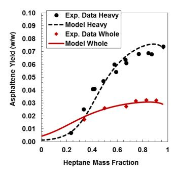
**Figure 8-8.** Asphaltene yield for heavy fraction and whole oil from in-situ converted oil 27034-113 diluted with n-heptane at 20°C and atmospheric pressure.
