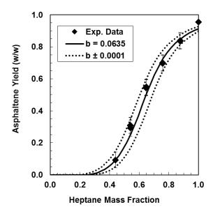
**Figure 5-26.** Fractional precipitation of WC-B-B2 asphaltenes in heptol solutions at  $20^{\circ}$ C and model results for  $b = 0.0635 \pm 0.0001$ .
