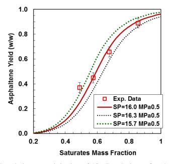
**Figure D.2.** Fractional asphaltene precipitation of 10 g/L solutions of asphaltenes from WC-C-B2 bitumen in toluene and saturates from 27034-113 at 21°C and atmospheric pressure and regular solution model predictions.
