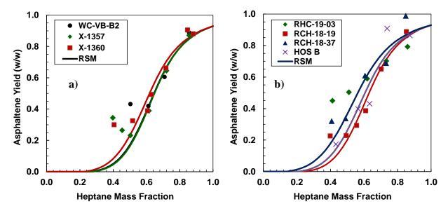
**Figure 6-12.** Measured and modeled fractional asphaltene precipitation of 10 g/L solutions of asphaltenes from WC-C-B2 bitumen in toluene and various aromatics from a) thermocracked and b) hydrocracked oils at 21°C and atmospheric pressure.
