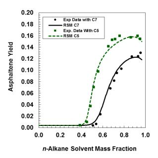
**Figure E.1.** Asphaltene yield and model results and predictions for Lloydminster crude oil diluted with n-heptane (black dots) and n-pentane and n-pentane (green squares) at 20°C. (Exp. Data from Akbarzadeh  $et\ al.\ (2005)$ ).
