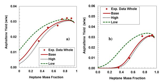
**Figure 8-11.** Asphaltene yield for whole crude oils diluted with n-heptane at 20°C: a) 27034-113 in-situ converted oil and b) Arabian medium oil at 20°C and atmospheric pressure using different enthalpy of vaporization correlations.
