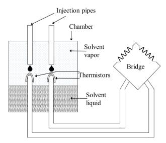
**Figure 3-6.** Schematic of a vapour pressure osmometer.
