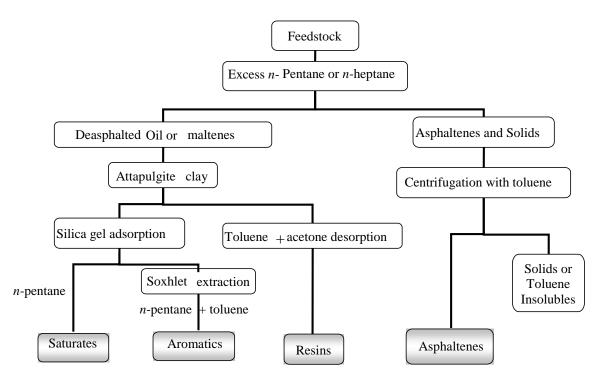
**Figure 3-5.** Schematic procedure of SARA fractionation.
