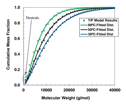
**Figure 5-9.** Self-association model results and fitted cumulative distribution with Eq. 5-1 for asphaltenes from WC-DB-A2.
