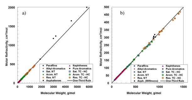
**Figure G-2.** Molar refraction of hydrocarbon fractions including asphaltenes using: a) associated molecular weight; b) monomer molecular weight.
