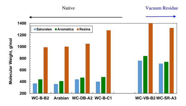
Figure 6-1. Molecular weight of SAR fractions from native oils and vacuum residues.
