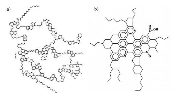
**Figure 2-3.** Hypothetical asphaltene structures: a) Archipelago: C<sub>412</sub>H<sub>509</sub>S<sub>17</sub>O<sub>9</sub>N<sub>7</sub> with a H/C ratio of 1.23 and a molecular weight of 6239 g/mol (Murgich *et al.*, 1999; Strausz *et al.*, 1992) b) Continent: C<sub>84</sub>H<sub>100</sub>N<sub>2</sub>S<sub>2</sub>O<sub>3</sub> with a H/C ratio of 1.19 and a molecular weight of 1276 g/mol (Dickie and Yen, 1967; Mullins, 2008).
