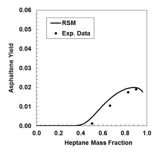
**Figure F.2**. Asphaltene yield for 27-168-179 whole crude oil diluted with n-heptane at 20°C: 1 at 20°C and atmospheric.
