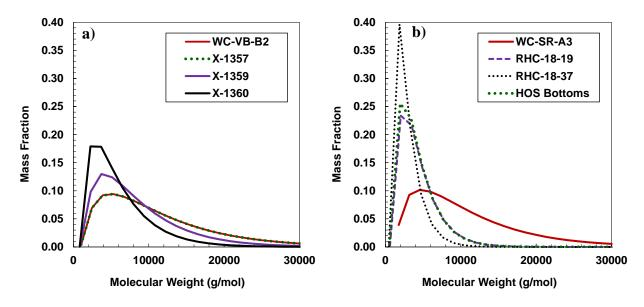
**Figure 5-4.** Molecular weight distribution at 50°C for asphaltenes from a) thermocracked and b) hydrocracked oils.
