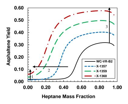
**Figure 7-8.** Asphaltene precipitation model predictions for thermocracked oils at 20°C. With higher conversion, the amount of TI increases (1), the onset shifts to lower concentrations (2), and the yield increases (3).
