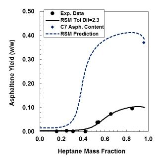
**Figure 7-5.** Asphaltene yield and model results for X-1357 (diamond) and toluene diluted X-1357 (circle) both diluted with n-heptane at  $20^{\circ}$ C.
