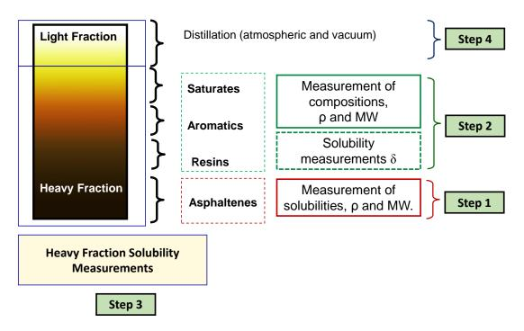
**Figure 1-1.** General methodology of the characterization and modeling of native and reacted oils applied in this thesis.
