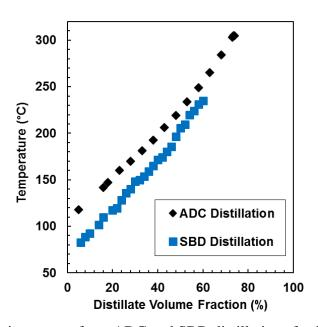
**Figure 3-2.** Distillation curves from ADC and SBD distillations for 27034-87 crude oil.
