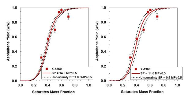
**Figure D.3.** Fractional asphaltene precipitation of 10 g/L solutions of asphaltenes from WC-C-B2 bitumen in toluene and saturates from X-1360 at 21°C and atmospheric pressure and regular solution model predictions with uncertainty of a)  $\pm 0.3$ MPa<sup>0.5</sup> and b)0.5MPa<sup>0.5</sup>.
