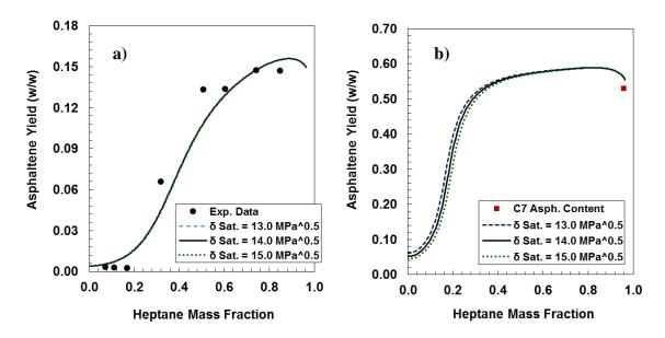
**Figure 7-11.** Asphaltene yield for X-1360 diluted with *n*-heptane a 20°C and effect of the saturates solubility parameter on the RSM results for: a) 2.3 w/w tol/oil dilution; b) predictions with no toluene dilution.
