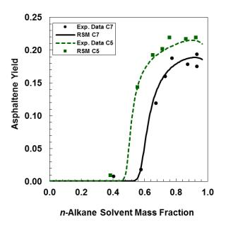
**Figure E.2.** Asphaltene yield and model results and predictions for Venezuela 2 crude oil diluted with n-heptane (black dots) and n-pentane and n-pentane (green squares) at 20°C. (Exp. Data from Akbarzadeh  $et\ al.\ (2005)$ ).
