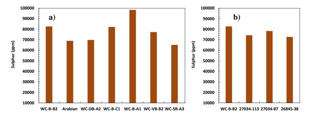
Figure 5-43. Sulphur content of asphaltenes from a) native and b) *in-situ* converted oils.
