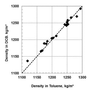
**Figure 3-11.** Comparison of densities measured in toluene and o-dichlorobenzene (DCB) for WC-VR-B2 and HOS Bottoms whole asphaltenes and their different solubility cuts. Data from Sadeghi –Yamchi (2014).
