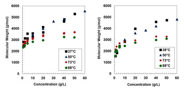
**Figure B.2**. Effect of temperature on molecular weight measurements for C7-asphaltenes from: a) X-1357; b) X-1359.
