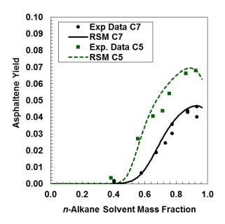
**Figure E.3.** Asphaltene yield and model results and predictions for Russia crude oil diluted with n-heptane (black dots) and n-pentane and n-pentane (green squares) at 20°C. (Exp. Data from Akbarzadeh  $et\ al.\ (2005)$ ).
