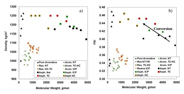
**Figure G-6.** a) Density at 20°C and b)FRI at 20°C as function of molecular weight for aromatics, resins and asphaltenes.
