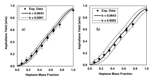
**Figure 5-27.** Fractional precipitation of HOS Bottoms asphaltenes in heptol solutions at 20°C and model results for a)  $b = 0.0643 \pm 0.0001$  and b)  $b = 0.0643 \pm 0.0002$ .
