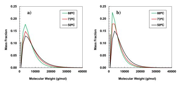
**Figure 5-13.** Effect of temperature in the molecular weight distribution of asphaltenes from a) X-1359 and b) X-1360 oil samples.
