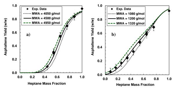
**Figure 5-31.** Fractional precipitation of asphaltenes in heptol solutions at 20°C and model results for a) WC-B-B2 with  $MW_A = 4500$  g/mol  $\pm$  10% and b)HOS bottoms with  $MW_A = 1200$  g/mol  $\pm$  10%.
