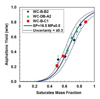
**Figure D.1.** Fractional asphaltene precipitation of 10 g/L solutions of asphaltenes from WC-C-B2 bitumen in toluene and various saturates from native at 21°C and atmospheric pressure and regular solution model predictions.
