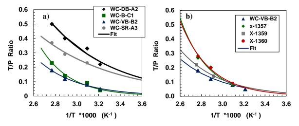
**Figure 5-14.** Temperature dependence of T/P ratio from the self-association model and fitted Equation. 5-5.
