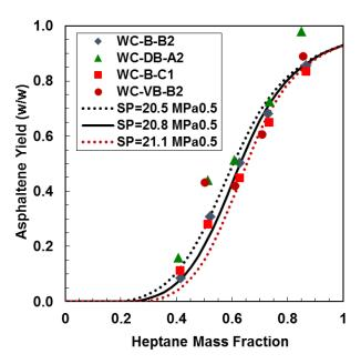
**Figure D.5.** Fractional asphaltene precipitation of 10 g/L solutions of asphaltenes from WC-C-B2 bitumen in toluene and various aromatics from native at 21°C and atmospheric pressure and regular solution model predictions.
