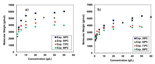
**Figure 5-5.** Effect of temperature in molecular weight measurements for asphaltenes from a) WC-DB-A2 and b) WC-VB-B2.
