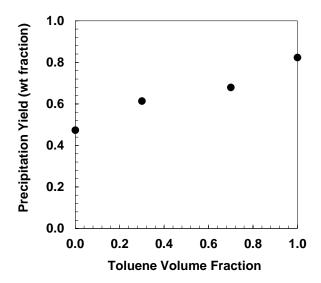
**Figure 5-46.** Fractional precipitation yield of toluene insoluble in a mixture of toluene and dichlorobenzene at 20°C and atmospheric pressure.
