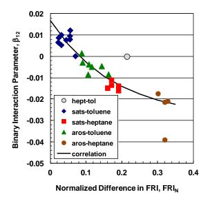
**Figure 3-12.** Relationship to normalized *FRI* of binary interaction parameters for the *FRI* of saturate and aromatic pseudo-binary mixtures with toluene and heptane (Okafor, 2013).
