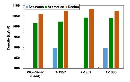
**Figure 6-7.** Density of SAR fractions from thermocracked oils and the feedstock at 20°C and atmospheric pressure. Note that for WC-VB-B2 and X-1359 there was not enough saturate sample to performed complete characterization.
