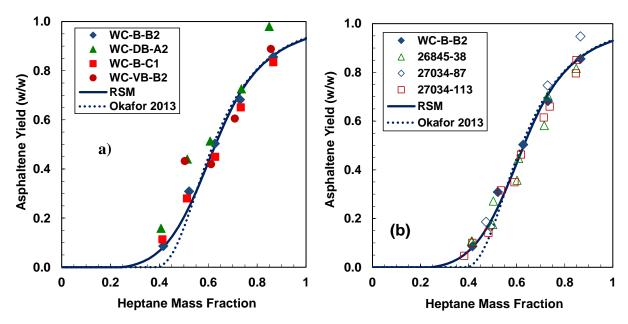
**Figure 6-11.** Fractional asphaltene precipitation of 10 g/L solutions of asphaltenes from WC-C-B2 bitumen in toluene and various aromatics from a) native and b) *in-situ* reacted oils at 21°C and atmospheric pressure.
