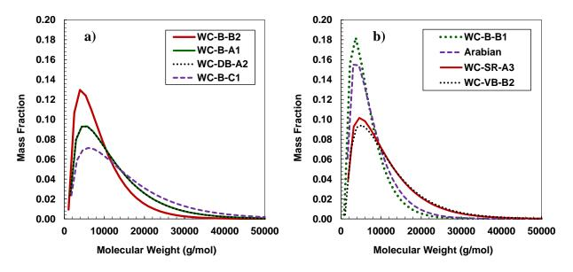
**Figure 5-2.** Molecular weight distribution at 50°C for asphaltenes from native oils.
