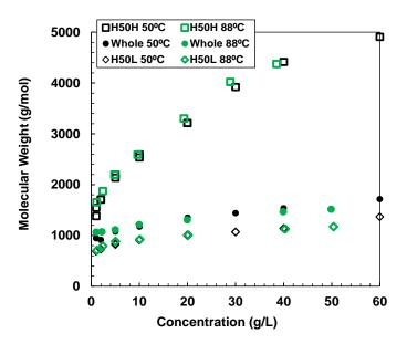
**Figure 5-7.** Temperature effect in molecular weight for asphaltene fractions from HOS Bottoms. H50H refers to the heavy (or precipitated) fraction from the precipitation experiment (solubility curve) with 50wt% heptol. H50L refers to the light (or soluble) fraction from the precipitation experiment (solubility curve) with 50wt% heptol.
