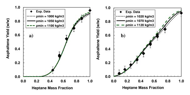
**Figure 5-32.** Fractional precipitation of asphaltenes in heptol solutions at 20°C and model results for a) WC-B-B2 with  $\rho_{min} = 1050 \pm 50 \text{ kg/m}^3$  and b) HOS bottoms with  $\rho_{min} = 1070 \pm 50 \text{ kg/m}^3$ .
