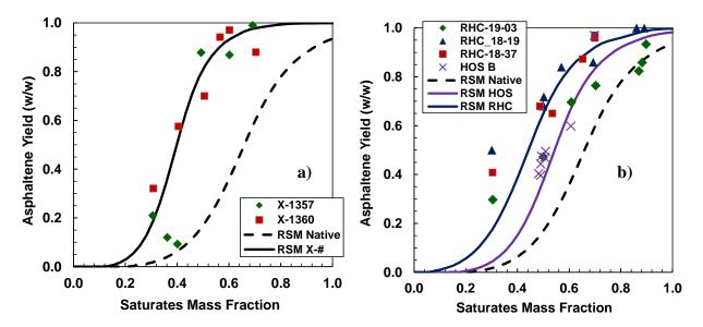
**Figure 6-10.** Measured and modeled fractional asphaltene precipitation of 10 g/L solutions of asphaltenes from WC-B-B2 bitumen in toluene and various saturates from a) thermocracked and b) hydrocracked oils at 21°C and atmospheric pressure.
