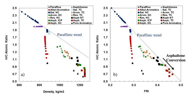
**Figure G-7.** H/C Atomic ratio as a function of density (a) and FRI (b) of hydrocarbon families and fractions.
