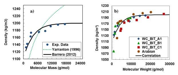
**Figure 4-1.** Density at 23°C as a function of molecular weight at 10 g/L for a) WC\_BIT\_A1 asphaltenes b) compared with density of asphaltene cuts from four samples at 23°C (Barrera *et al.* 2013).
