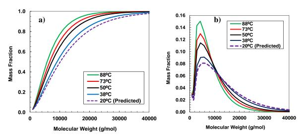
**Figure 5-15.** a) Cumulative and b) discrete molecular weight distribution with temperature and prediction at 20°C.
