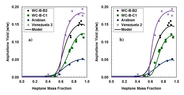
**Figure 7-1.** Asphaltene yield for crude oils diluted with n-heptane at  $20^{\circ}$ C: a) solubility parameter calculated with tuned b for each crude oil asphaltenes; b) solubility parameter calculated with average b for native oils (b=0.0634).
