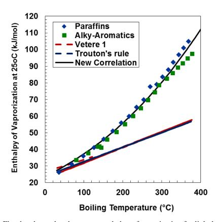
Figure 8-4. Fitted and correlated apparent enthalpy of vaporization for light hydrocarbons.
