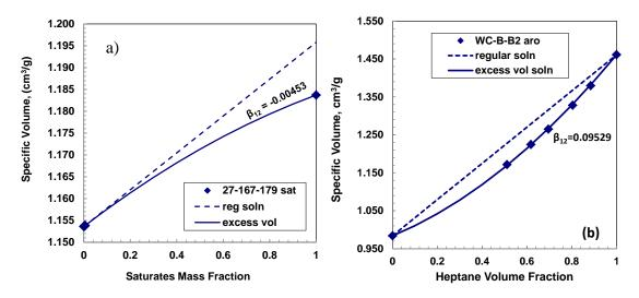
**Figure 3-9.** Density measurements of a) 27-168-179 saturates in toluene b) WC-B-B2 aromatics with heptane. Data from Okafor (2013). Note, Figure 3-9a a low concentration contain at least four data points which are not visible at the scale of the plot.
