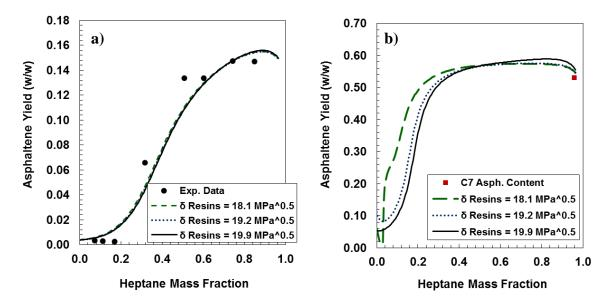
**Figure 7-15.** Asphaltene yield of X-1360 diluted with n-heptane at 20°C and effect of lower solubility parameter of resins on the model results for: a) toluene diluted sample; b) no toluene dilution.
