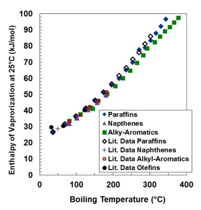
**Figure 8-3.** Apparent enthalpy of vaporization (solid symbols) and actual enthalpy of vaporization data from the literature at standard conditions (open symbols) versus boiling point for different chemical families.
