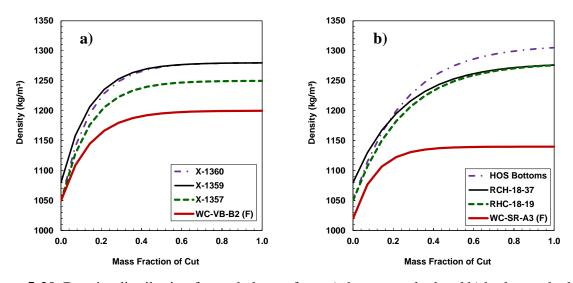
Figure 5-20. Density distribution for asphaltenes from a) thermocracked and b) hydrocracked oils.
