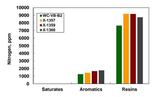
Figure 6-21. Nitrogen content in SAR fractions from thermocracked oils and the feedstock.
