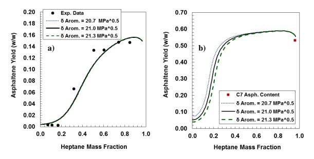
**Figure 7-13.** Asphaltene yield for X-1360 diluted with n-heptane a 20°C and effect of the aromatics solubility parameter on the RSM results for: a) 2.3 w/w tol/oil dilution; b) predictions with no toluene dilution.
