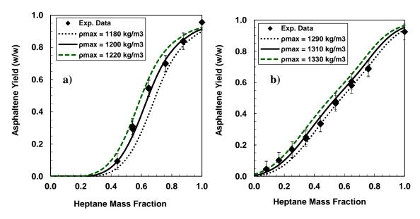
**Figure 5-33.** Fractional precipitation of asphaltenes in heptol solutions at 20°C and model results for a) WC-B-B2 with  $\rho_{max} = 1200 \pm 20$  kg/m<sup>3</sup> and b) HOS bottoms with  $\rho_{max} = 1310 \pm 20$  kg/m<sup>3</sup>.
