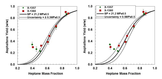
**Figure D.6.** Fractional asphaltene precipitation of 10 g/L solutions of asphaltenes from WC-C-B2 bitumen in toluene and aromatics from X-1357 and X-1360 at 21°C and atmospheric pressure and regular solution model predictions with uncertainty of a)  $\pm 0.3$ MPa<sup>0.5</sup> and b)0.5MPa<sup>0.5</sup>.
