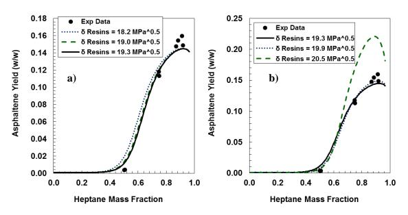
**Figure 7-14.** Asphaltene yield for WC-B-B2 diluted with *n*-heptane at 20°C and effect of uncertainty in the solubility parameter of resins on the model results for: a) lower values; b) higher values of the solubility parameter than given by the correlation for native oils.
