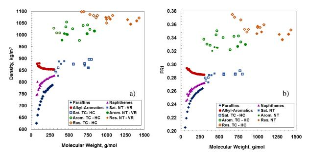
**Figure G-5.** a) Density at 20°C and b) refractive index at 20°C as function of molecular weight of different hydrocarbon families/fractions.
