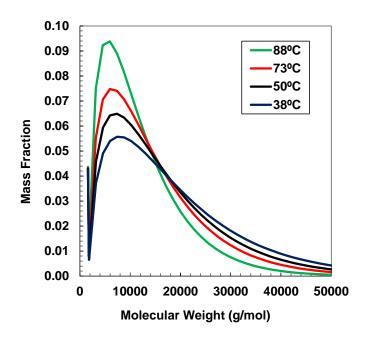
**Figure 5-11.** Effect of temperature in the molecular weight distribution of asphaltenes from WC-B-C1.
