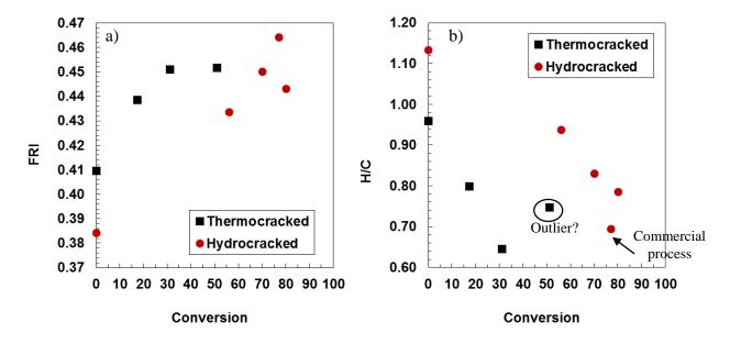
**Figure G-8.** FRI (a) and atomic H/C ratio (b) as a function of conversion for asphaltenes from thermocracked and hydrocracked samples.
