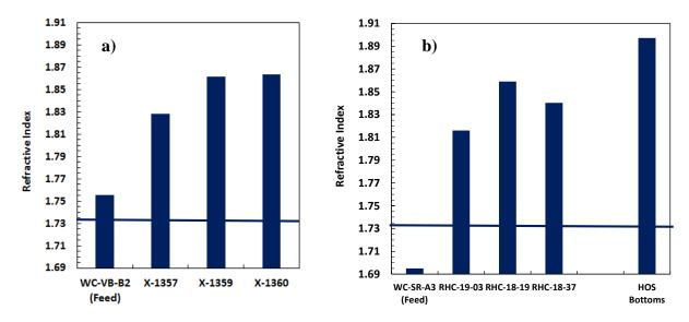
**Figure 5-38.** Refractive index comparison of asphaltenes from a) thermocracked and b) hydrocracked oils at 20°C and atmospheric pressure.
