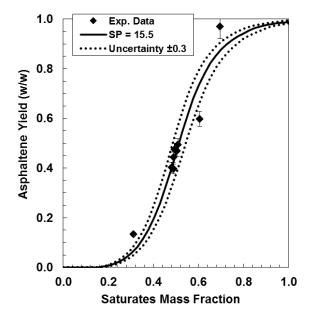
**Figure D.4.** Fractional asphaltene precipitation of 10 g/L solutions of asphaltenes from WC-C-B2 bitumen in toluene and saturates from HOS Bottoms at 21°C and atmospheric pressure and regular solution model predictions.
