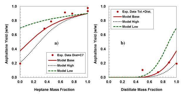
**Figure 8-5.** Measured and modeled asphaltene yield from mixtures of asphaltenes in: a) distillate+heptane; b) toluene+distillate; destillate from 27034-87 *in situ* converted oil and WC-B-B2 C7 asphaltenes.
