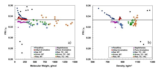
**Figure G-3**. FRI to density ratio for pure hydrocarbons and SAR fractions. Line indicates the "one-third-rule".
