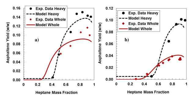
**Figure 8-9.** Asphaltene yield for heavy fraction and whole oil from in-situ converted oils 26845 (a) and 27034-87 (b) diluted with n-heptane at 20°C and atmospheric pressure.
