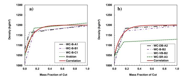
**Figure 5-18.** Density distribution for asphaltenes from native oils at 20°C and atmospheric pressure. Lines in Figures are previous density distributions fitted by Barrera et al (2013) for asphaltene from each specific native sample. The density distribution used two linear correlations (Barrera 2012, Barrera *et al.* 2013).
