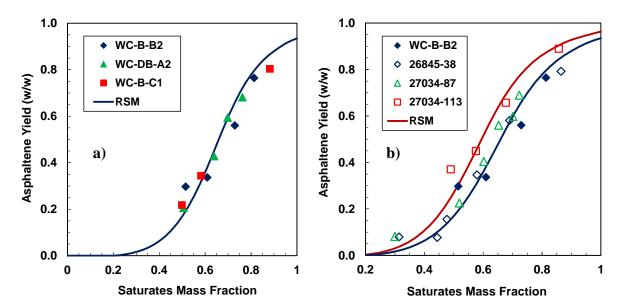
**Figure 6-9.** Fractional asphaltene precipitation of 10 g/L solutions of asphaltenes from WC-B-B2 bitumen in toluene and various saturates from a) native and b) *in-situ* reacted oils at 21°C and atmospheric pressure and regular solution model predictions.
