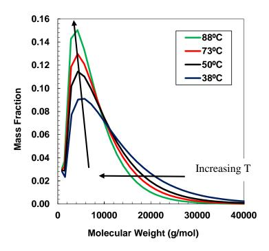
**Figure 5-10.** Effect of temperature in the molecular weight distribution of asphaltenes from WC-DB-A2.
