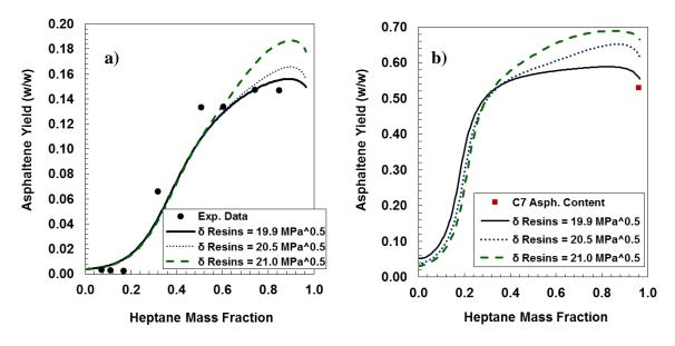
**Figure 7-16.** Asphaltene yield of X-1360 diluted with n-heptane at 20°C and effect of higher solubility parameter of resins on the model results for: a) toluene diluted sample; b) no toluene dilution.
