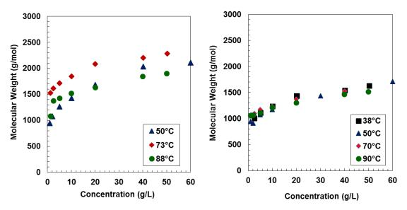
**Figure B.3**. Effect of temperature on molecular weight measurements for C7-asphaltenes from: a) RHC-18-19; b) HOS Bottoms.
