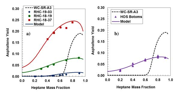
**Figure 7-9.** Asphaltene yield for hydrocracked oils diluted with n-heptane at 20°C a) RHC samples b) HOS bottoms.
