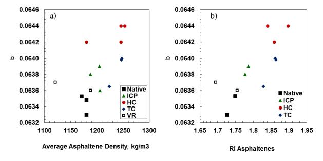
**Figure G-12.** Parameter b as function of: a) the average asphaltene density; b) refractive index.
