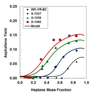
**Figure 7-4.** Asphaltene yield for toluene-diluted-thermocracked oils (2.3 g tol/g oil) diluted with n-heptane at 20°C.
