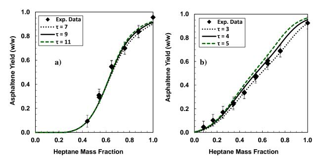
**Figure 5-35.** Fractional precipitation of asphaltenes in heptol solutions at 20°C and model results for a) WC-B-B2 with  $\tau = 9 \pm 2$  and b) HOS bottoms with  $\tau = 4 \pm 1$  kg/m<sup>3</sup>.
