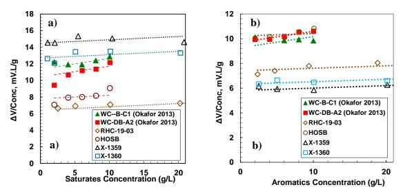
**Figure 3-8.** VPO measurements for a) saturate and b) aromatic fractions in toluene at 50°C.
