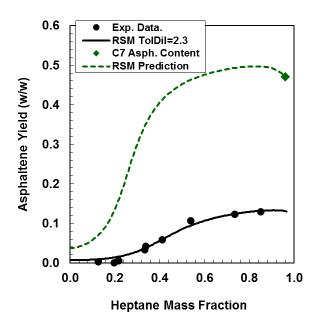
**Figure 7-6.** Asphaltene yield and model results for X-1359 (diamond) and toluene diluted X-1359 (circle) both diluted with n-heptane at 20°C.
