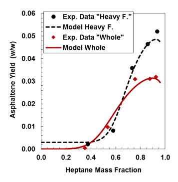
**Figure 8-7.** Asphaltene yield for heavy fraction and whole oil from Arabian medium oil diluted with n-heptane at 20°C and atmospheric pressure. Note, the whole oil contains 0.3 wt% toluene insolubles.
