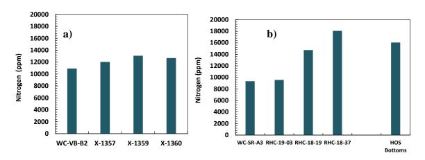
Figure 5-42. Nitrogen content of asphaltenes from a) thermocracked and b) hydrocracked oils.
