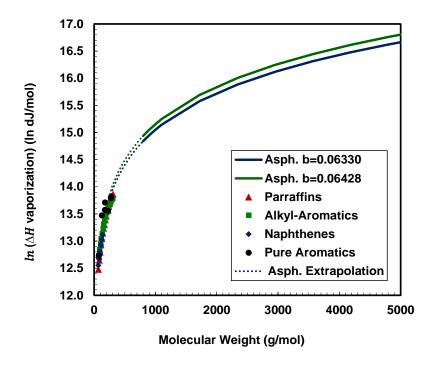
Figure 5-21. Extrapolation of the enthalpy of vapourization correlation.
