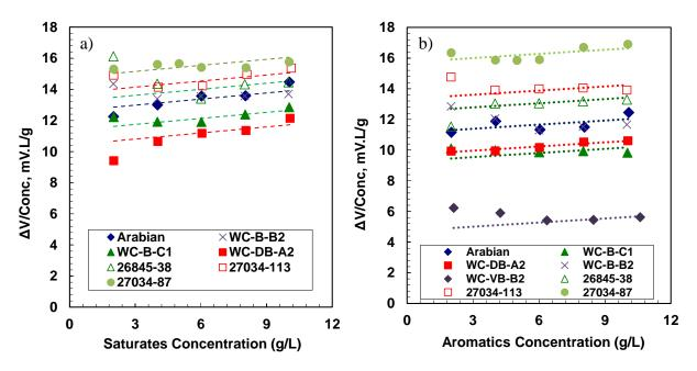
**Figure 3-7.** Measurements from the VPO for a) saturates and b) aromatics in toluene at 50°C.
