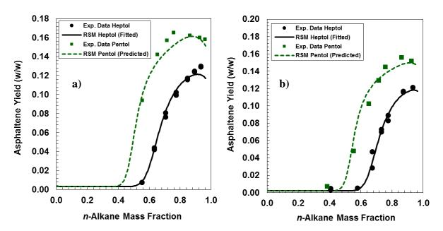
**Figure 7-2.** Asphaltene yield and model results and predictions for Cold Lake (a) and Venezuela 1 (b) crude oils diluted with n-heptane (black dots) and n-pentane (green squares) at 20°C. Solubility parameter calculated with average b for native oils.
