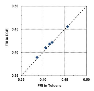
**Figure 3-17.** Comparison of *FRI* of Asphaltenes calculated from Rm from toluene and DCB solutions at 20°C and atmospheric pressure using average monomer molecular weight.
