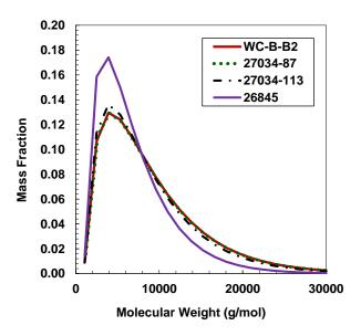
**Figure 5-3.** Molecular weight distribution at 50°C for asphaltenes from *in-situ* converted oils.
