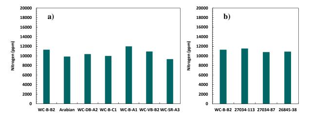
**Figure 5-41.** Nitrogen content of asphaltenes from a) native and b) *in-situ* converted oils.
