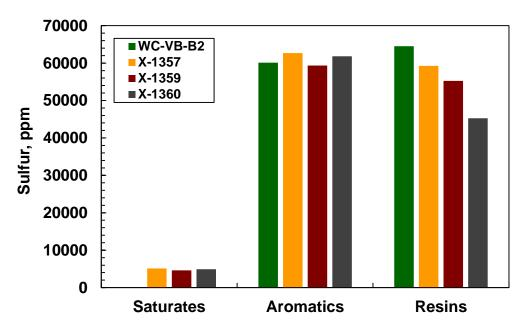
Figure 6-19. Sulfur content in SAR fractions from thermocracked oils and the feedstock.
