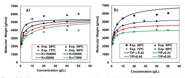
**Figure 5-8.** Effect of a) the association constant, K, and b) T/P ratio in the self-association model.
