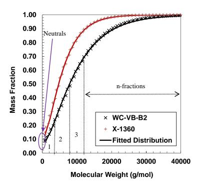
**Figure 5-1.** Schematic representation of the distribution discretization.
