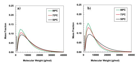
**Figure 5-12.** Effect of temperature in the molecular weight distribution of asphaltenes from a)WC-VB-B2 and b) X-1357 oil samples.
