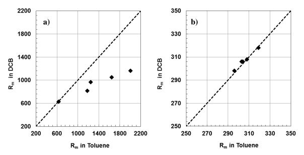
**Figure 3-16.** Comparison of the molar refractivity of asphaltenes in toluene and DCB solutions at 20°C and atmospheric pressure using: a) associated molecular weight; b) average monomer molecular weight.
