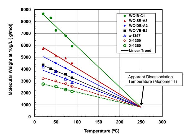
**Figure 5-17.** Linear temperature dependence and average apparent disassociation temperature for the molecular weight of Asphaltenes from native and reacted oils.
