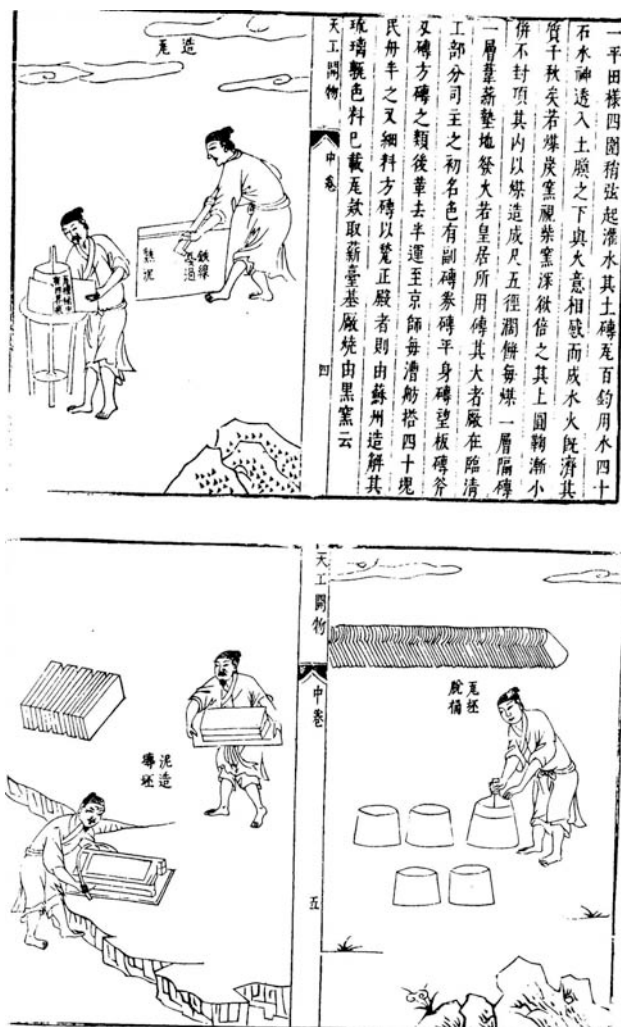
Figure 10. Tiangong kaiwu woodblock illustrations: making tiles, making bricks, removing tiles from moulds.
