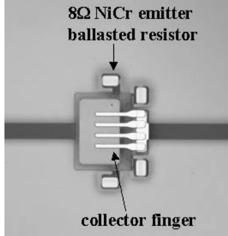
Figure 4.8: 4-finger 1\ \mu\text{m} \times 16\ \mu\text{m} common emitter TS DHBT
