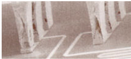
Figure A.6.9: SEM photograph of high rate plating failure
