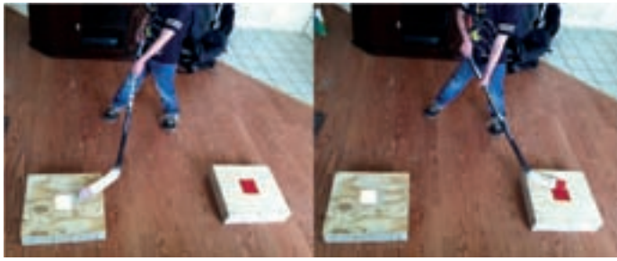
Image 1: Study participant performing test with a left hockey stick (stick held to the left of his body). He alternates back and forth between hitting the white target on the box to his right and the red target on the box to his left. Notice the extreme supination and pronation of his top hand (right hand). The test is designed to mimic the supination and pronation and back and forth motions used while playing hockey.
