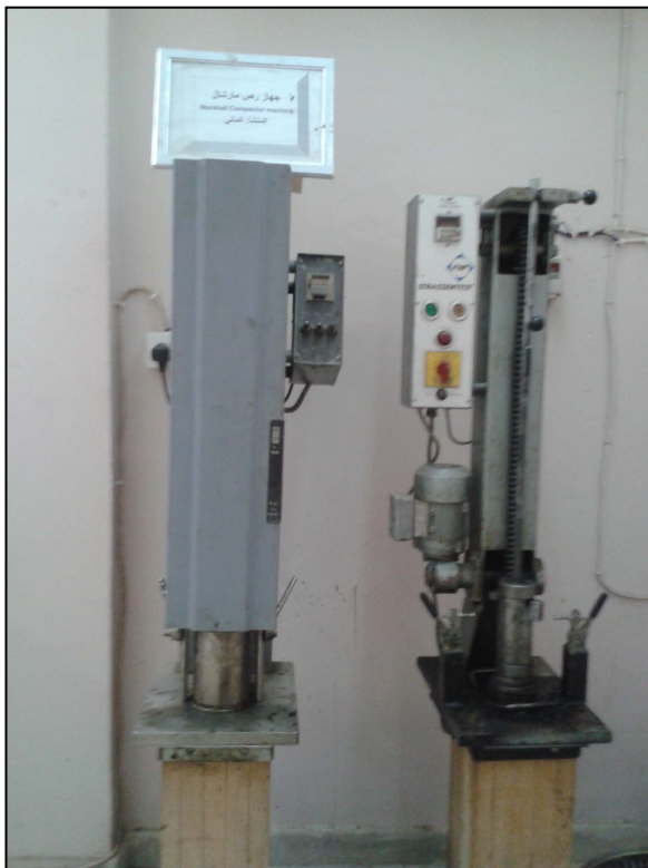
Figure (8-3) Compaction hammer & Marshall apparatus
