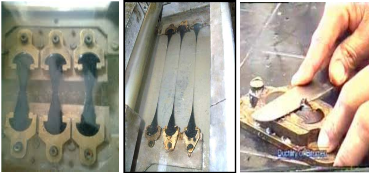
Figure (2-1) Ductility testing machine
