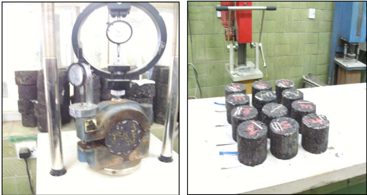
Figure (8-6) Marshall test
