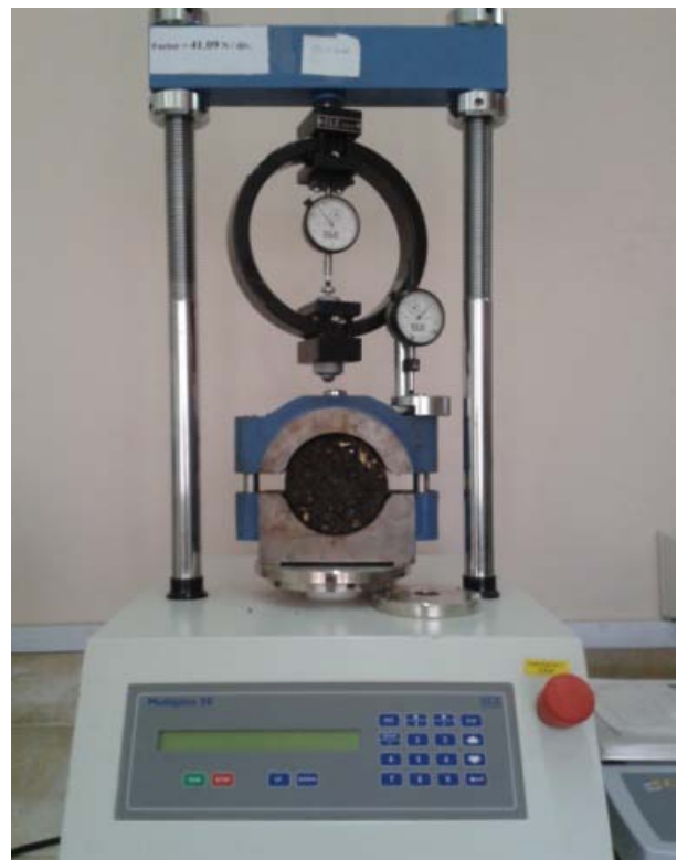
Figure (8-3) Compaction hammer & Marshall apparatus
