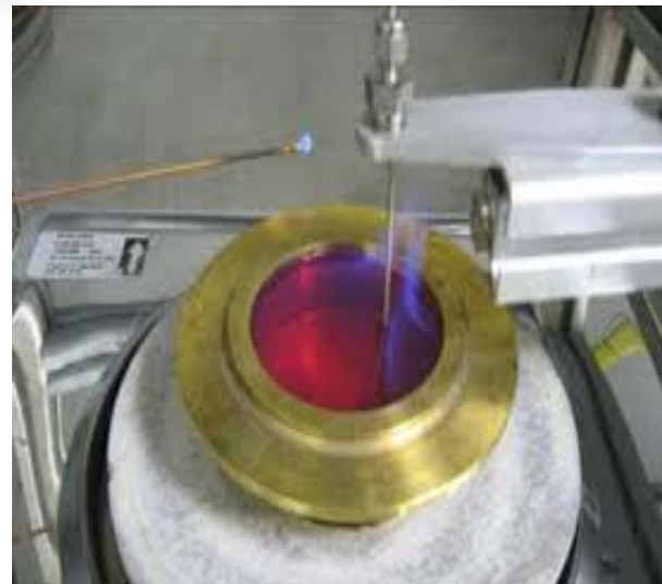
Figure (6-2) Burning the surface of the sample
