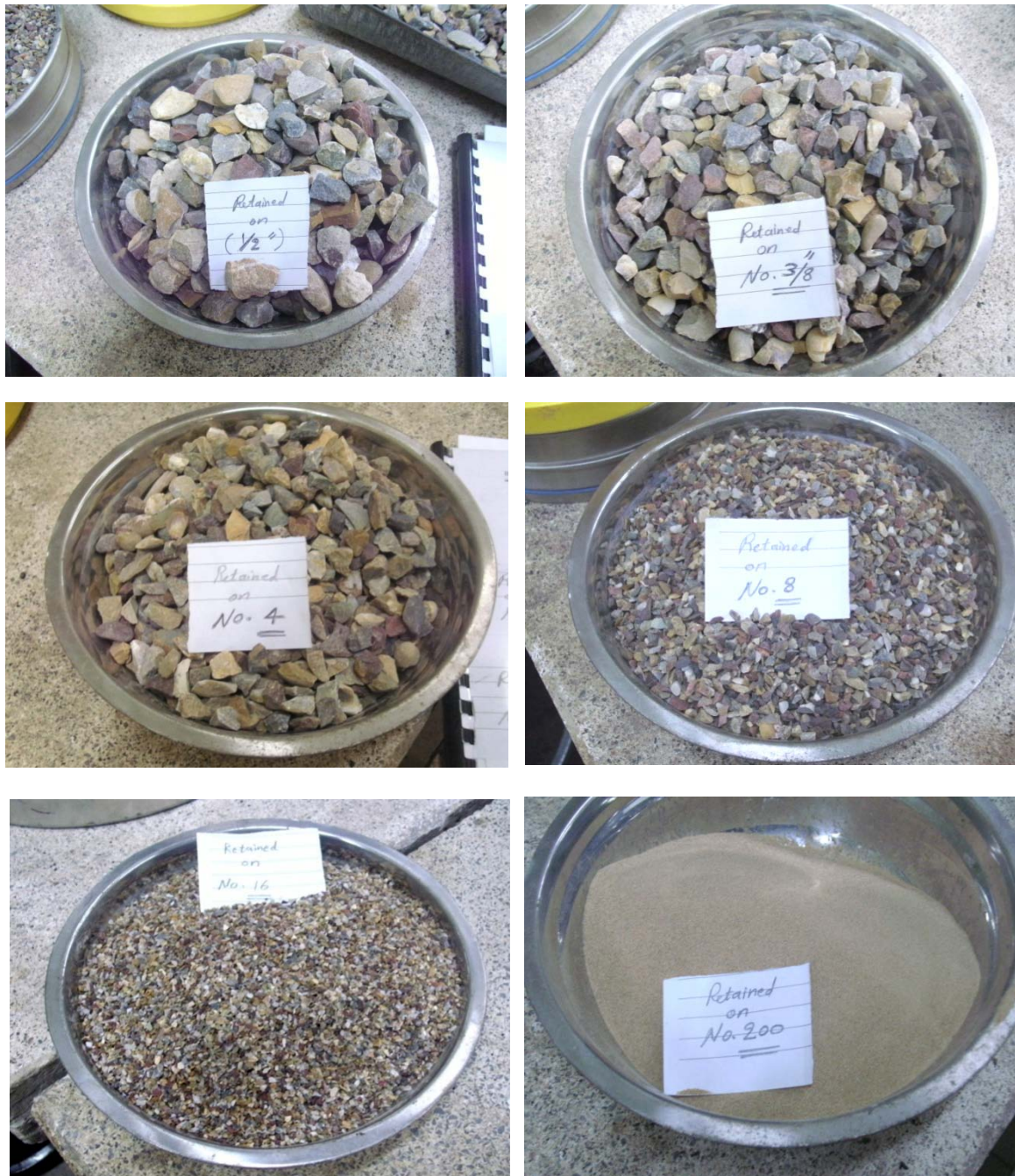
Figure (8-4) Separated aggregate by dry sieving into the desired size fractions
