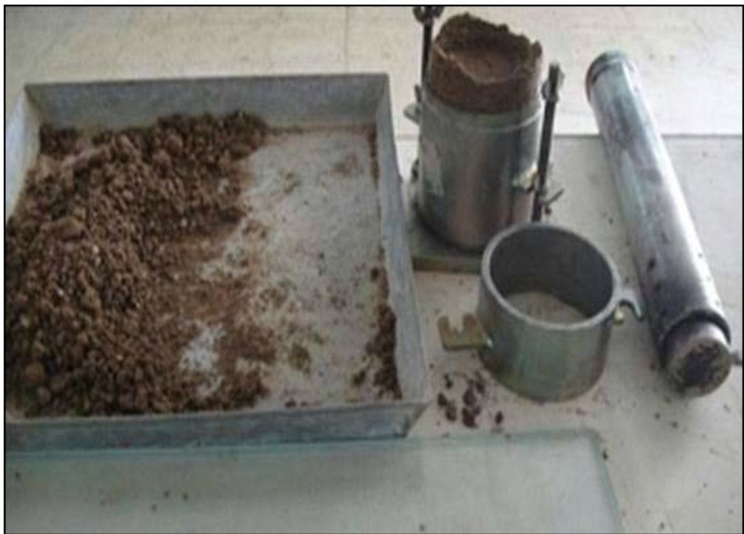
Figure (7-1) Molds of California Bearing Ratio Test apparatus
