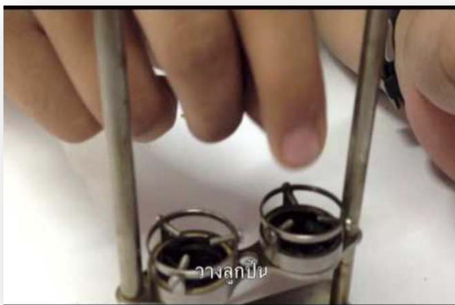
Figure (4-1) Softening point device
