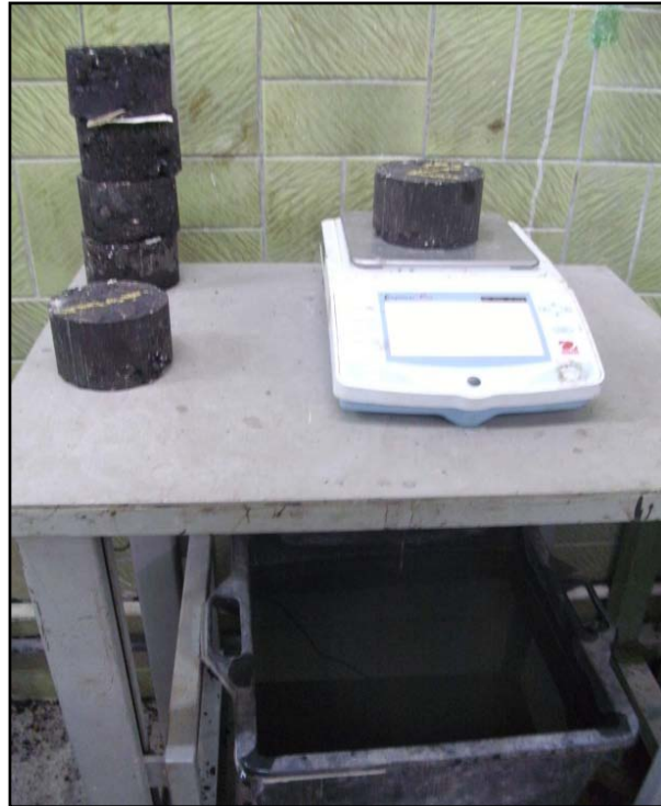
Figure (8-1) Water tank balance
