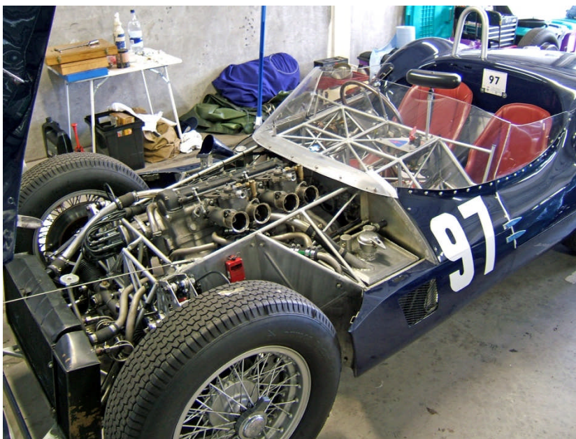
Image 5 – A space frame from a Maserati Tipo 61
