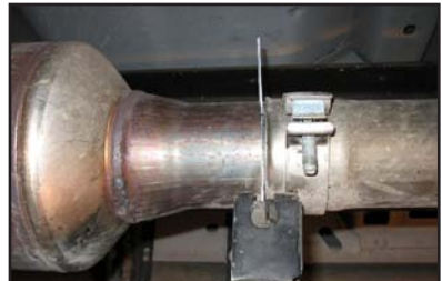
#2 Cut Exhaust in front of band clamp
