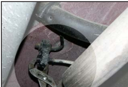
#7 Remove necessary exhaust hangers
