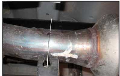
#3 Cut in front of Catalytic Converter
