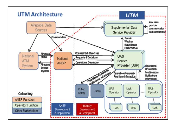
In this example of a federated architecture, there is still one central regulator, functionally the same as for the centralized model. Similarly, in this example, there is also a single State ANSP. The difference comes in the relationship between the regulator, the ANSP and the USPs.
