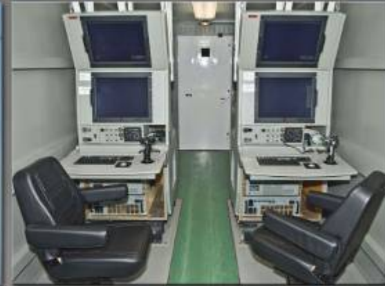
VTUAV Control Station Integrated Into the Ship's Combat Information Center
