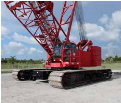
Manitowoc 14000 220 Ton Self-Erecting Orlando, FL, USA
