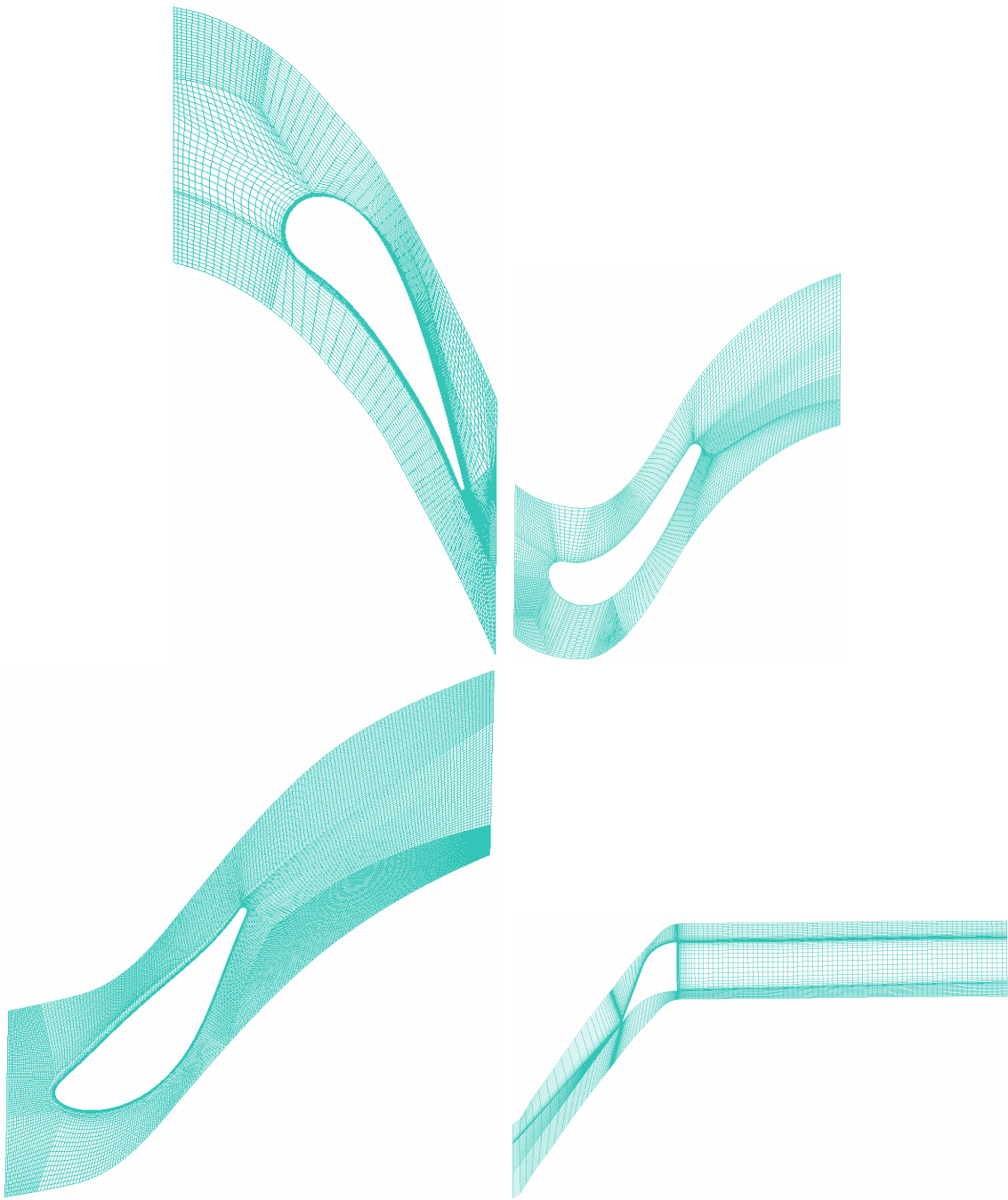
Figure 12: From upper left to lower right: stator, rotor, TMS and deswirler.
