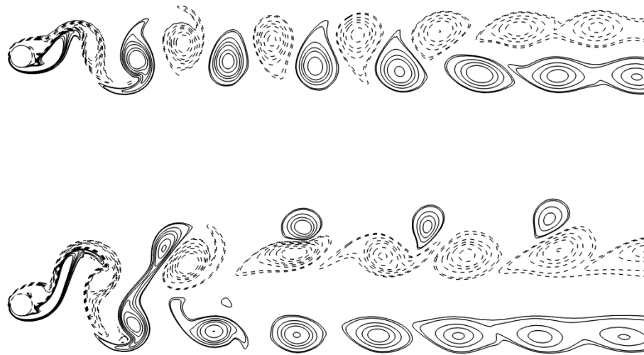
Fig.2.4 Wake structure showing (2S) Karman vortex shedding mode for low amplitude A=0.199 (top) and P+S shedding mode for A=0.696 (bottom)
