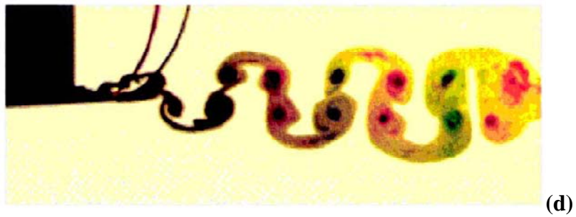
Fig.2.7 Wake comparison at k=7.86 and a) h = 0.02 b) h = 0.025 c) h = 0.03 d) experimental dye visualization for h = 0.02
