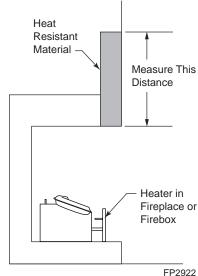
Figure 4 -Measure Heat Resistant Material
