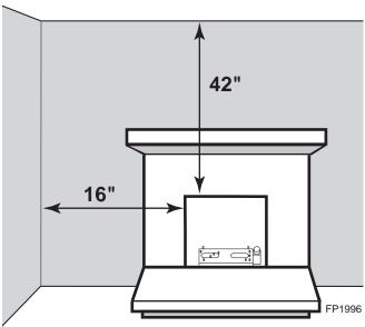
Figure 3 -Sidewall and Ceiling Clearances
