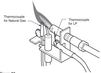
Figure 30 - Correct Pilot Flame Appearance
