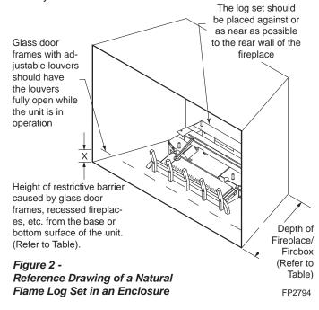
The dimensions shown in Figures 3 through 11 and defined in the fireplace manufacturer's instructions are *minimum clearances* to maintain when installing this heater. Left and right clearances are determined when facing the front of the heater.
