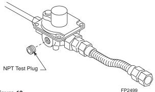
Figure 13 -Manual Control Pressure Test Point Location
