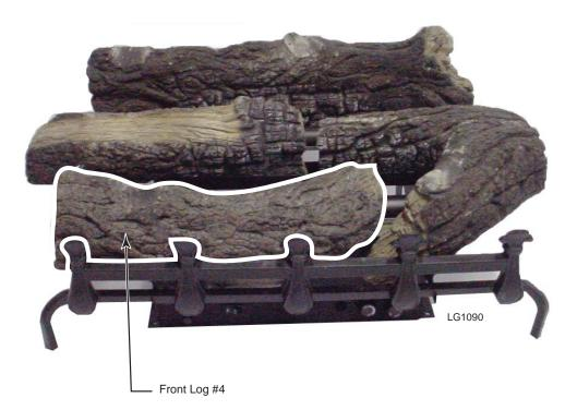
4. Place Front Log (#4) in between burner and grate so that notched areas fit between grate supports. *Figure 22*
