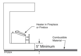
Figure 8 - Minimum Clearance Above Combustible Flooring
