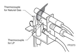
Figure 29 - Incorrect Pilot Flame Appearance
