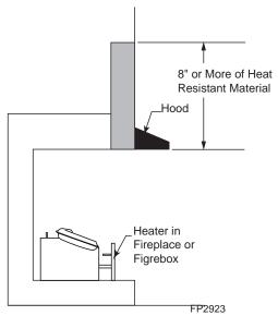
Figure 5 -Measure Heat Resistant Material for Mantel
