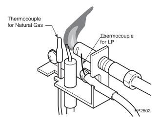
Figure 31 - Incorrect Pilot Flame Appearance
