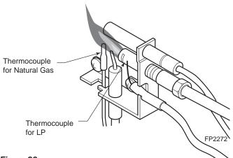
Figure 28 - Correct Pilot Flame Appearance
