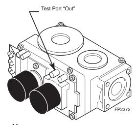
Figure 14 -Millivolt Control Pressure Test Point Location
