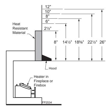
Figure 6 - Minimum Mantel Clearance with Hood
