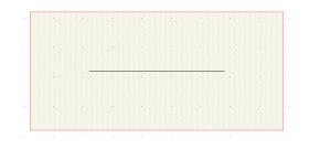
The small black line shows the actual starting and ending points the user selected. However, due to the fact that the line width was set at 1 micron, the computer adds .5 microns to all sides of your drawn line. Keep this in mind when you are trying to line up lines with other objects.
