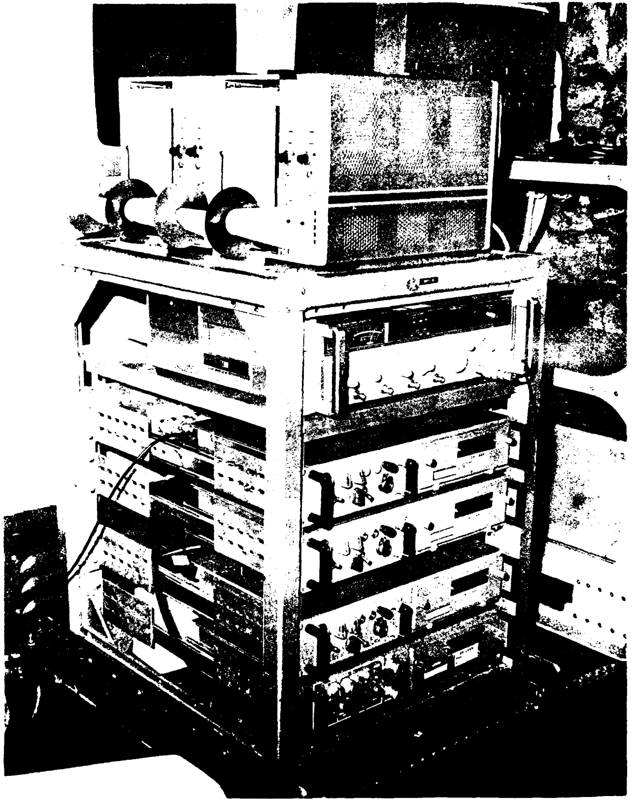
Figure 4-3. FAATC Signal Strength Measurement Receivers, Strip Chart Recorders, and Signal Standard.
