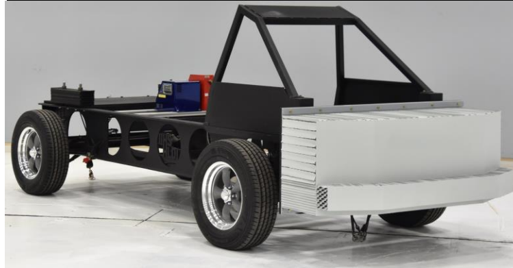
1,900 kg cart w/suspension MDB 2.0 barrier face
