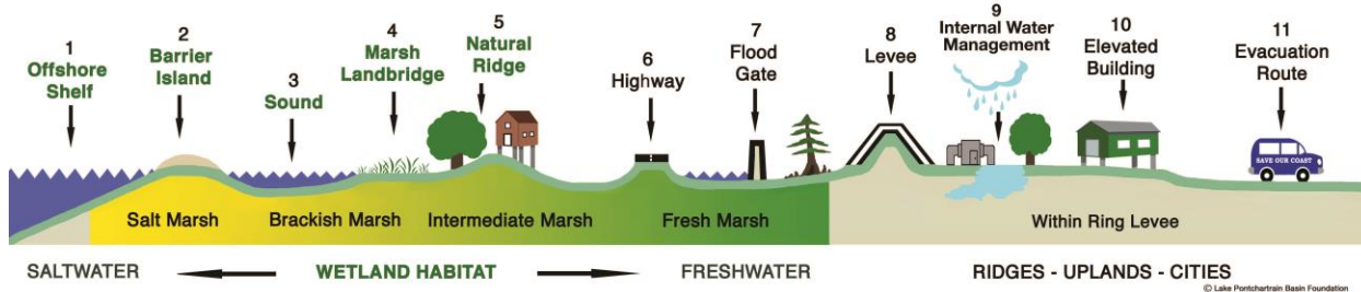
Figure 3: The Multiple Lines of Defense Strategy showing how healthy swamps reinforce flood protection levees by absorbing storm surge energy.
