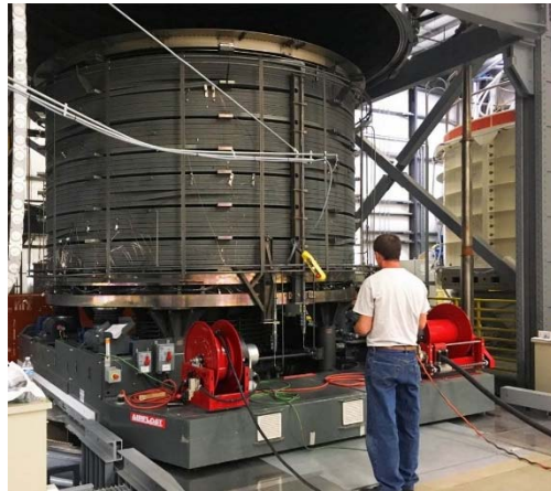
Central Solenoid Module 1 after completing heat treatment at General Atomics Poway, CA facility
